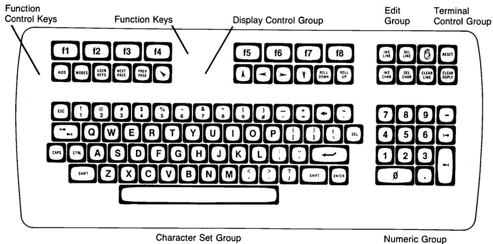
Figure D-25. HP2625A and HP2628A Keyboard
