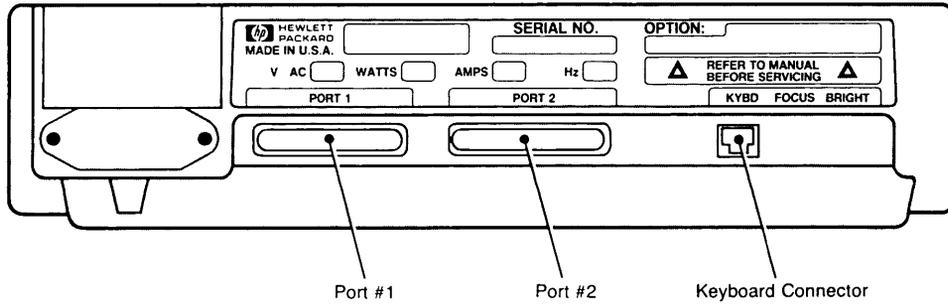
Figure D-24. HP2625A and HP2628A Rear View
