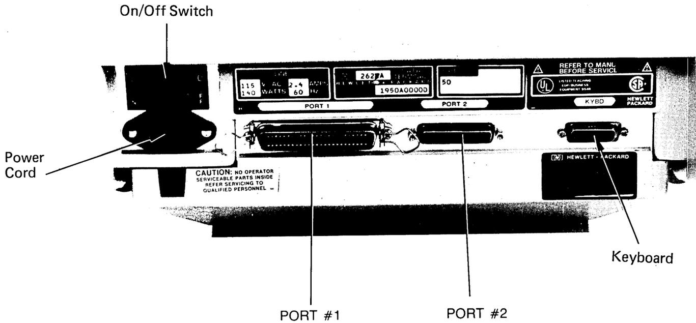
Figure D-22. HP2623A and HP2627A Rear View
