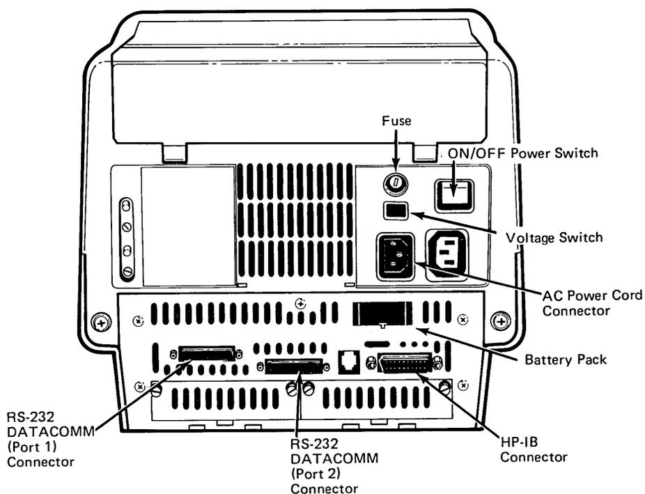
Figure D-27. HP 150 Rear View
