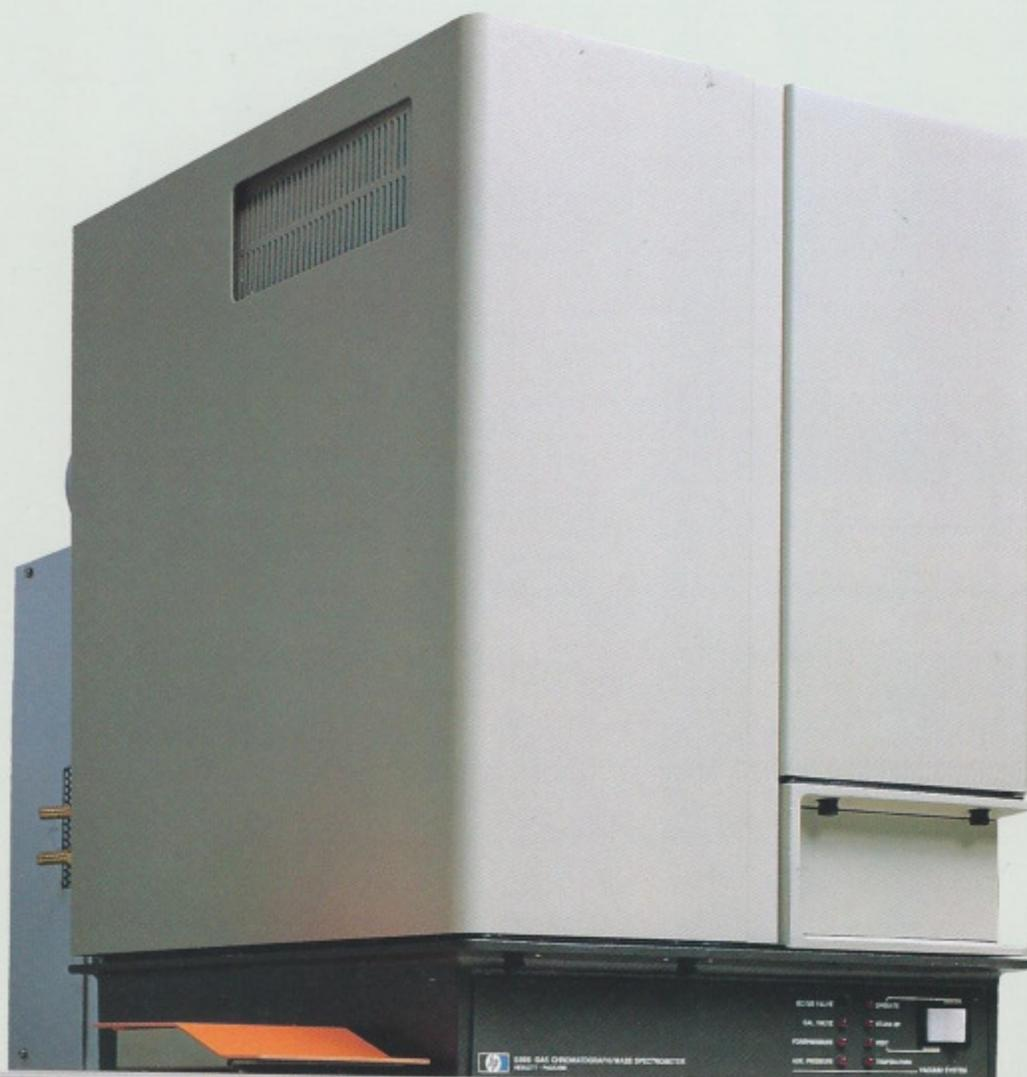
HP 5995C has a standard capillary split/splitless injector and a choice of two interfaces between the column and the ion source.
