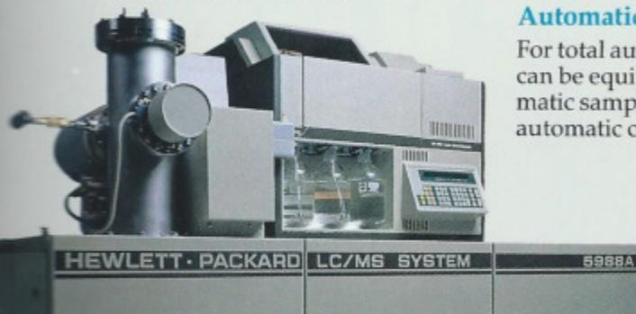
The HP 5988A can be an LC/MS. You can buy it without GC and add your own liquid chromatograph or the HP 1090 LC as shown here.
