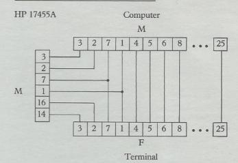
Pins 4, 5, 6 and 8 through 25 are directly connected between the computer and terminal connectors.
