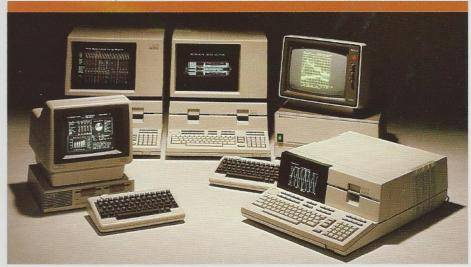
For engineering or scientific calculations which require 16/32-bit speed and data-handling capabilities, Series 200 computers in stand-alone configurations offer you low-cost, reliable performance. When combined with the Series 500, they can serve as the "low end" performance in a complete workstation-mainframe configuration — for example, a
