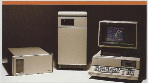
any Series 500 model can have up to 2.5 Mbytes internal memory.
