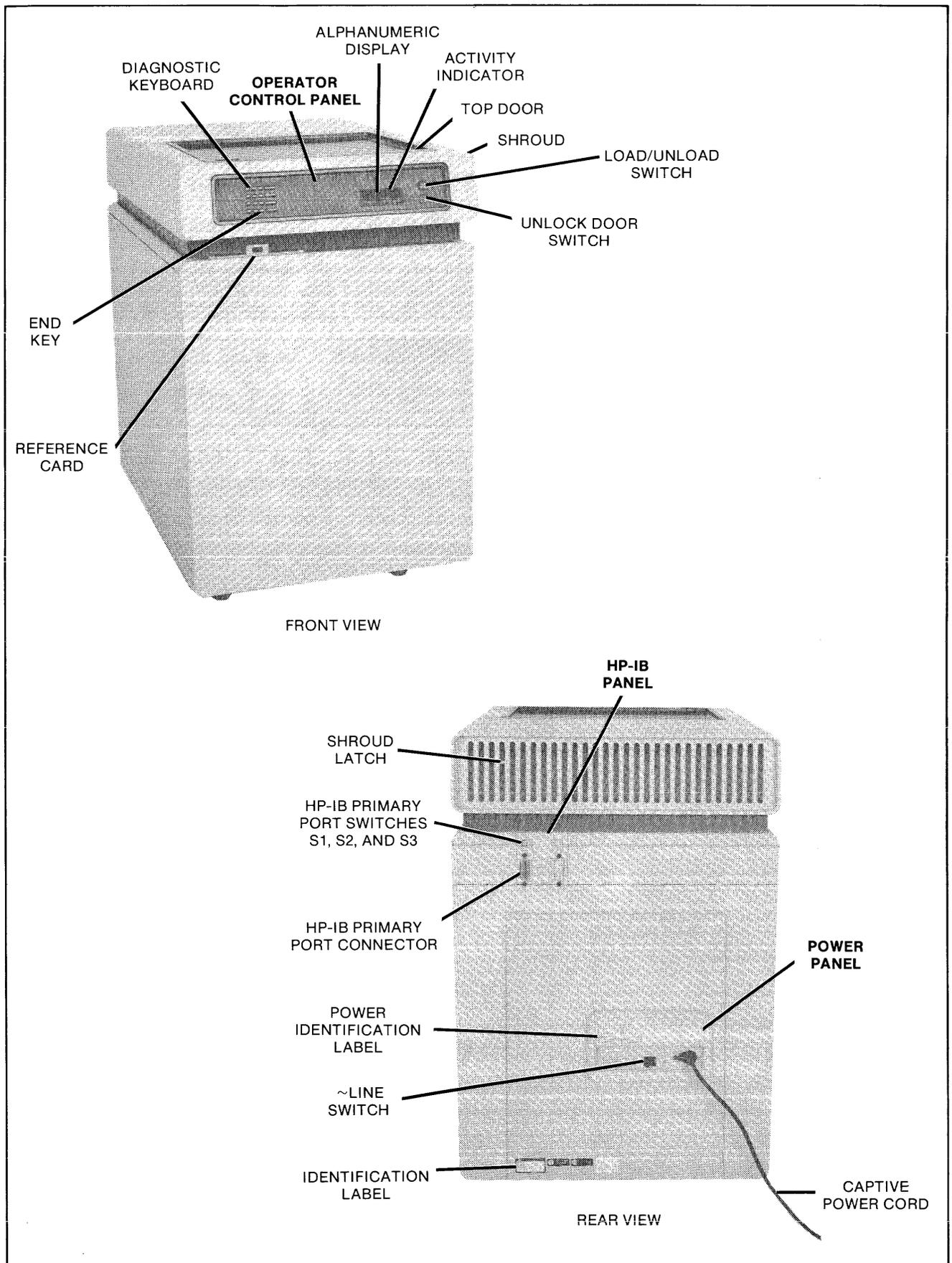
Figure 3-1. Switches, Indicators, and Connectors
