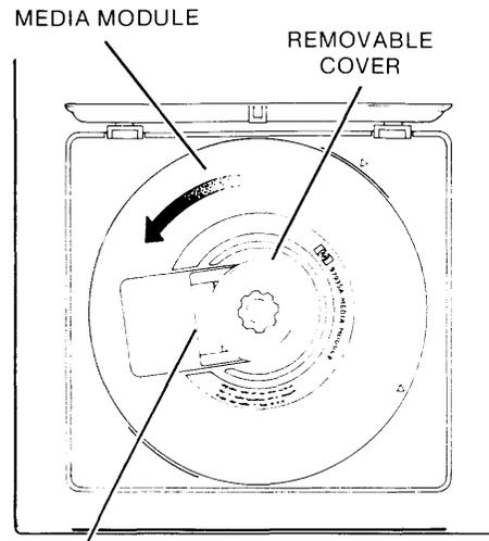
2. USING BOTH HANDS, ROTATE THE MEDIA MODULE COUNTERCLOCKWISE UNTIL THE INDEXING MARKS ARE ALIGNED AS SHOWN OPPOSITE. WHEN PROPERLY ALIGNED, LIFT THE MEDIA MODULE FROM THE MODULE CHAMBER.
