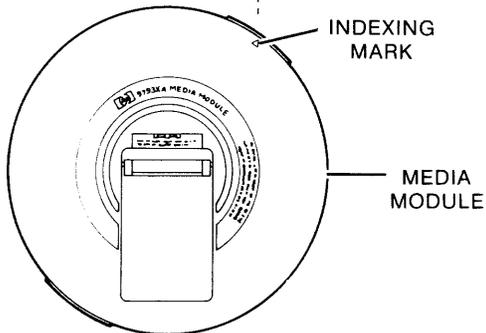
2. HOLDING THE MEDIA MODULE BY THE RAISED HANDLE, ALIGN THE INDEXING MARK ON THE MEDIA MODULE WITH THE INDEXING MARK ON THE MODULE CHAMBER, AS SHOWN OPPOSITE. WHEN PROPERLY ALIGNED, LOWER THE MEDIA MODULE INTO THE MODULE CHAMBER.
