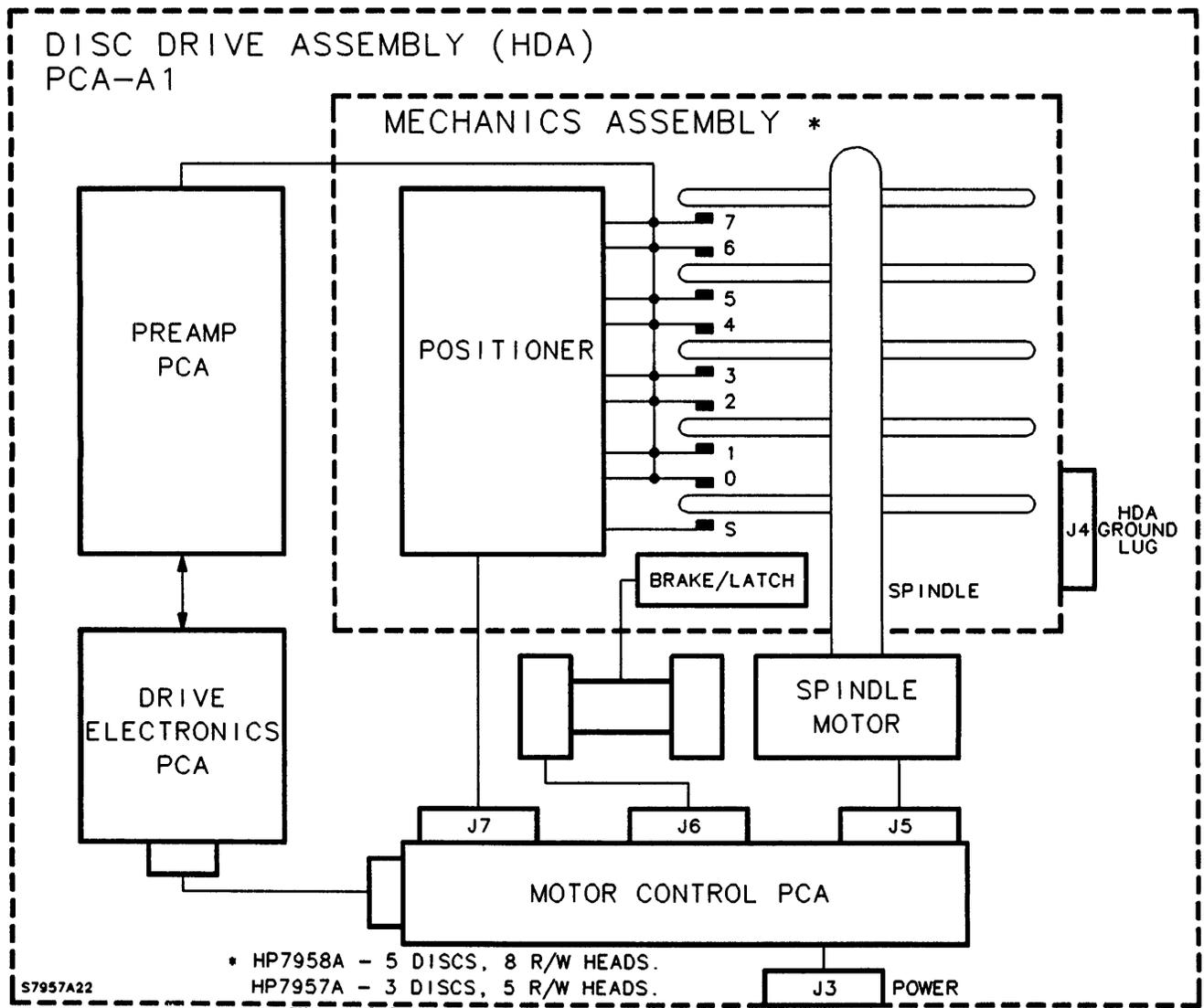
Figure 3-3. Disc Drive Assembly PCA-A1 Block Diagram
