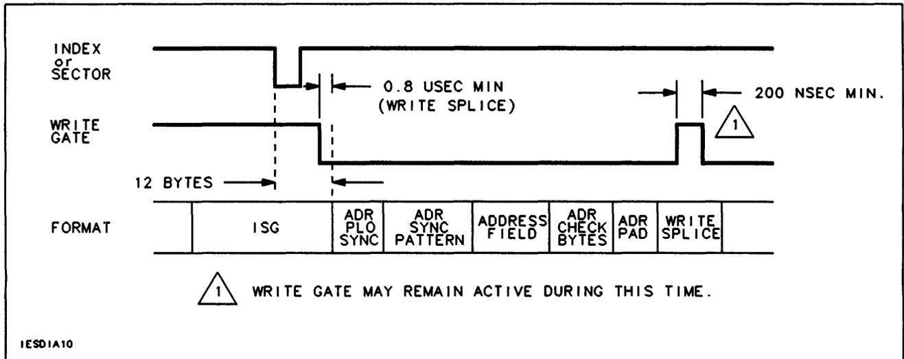
Figure 2-2. Write Gate Timing During Format
