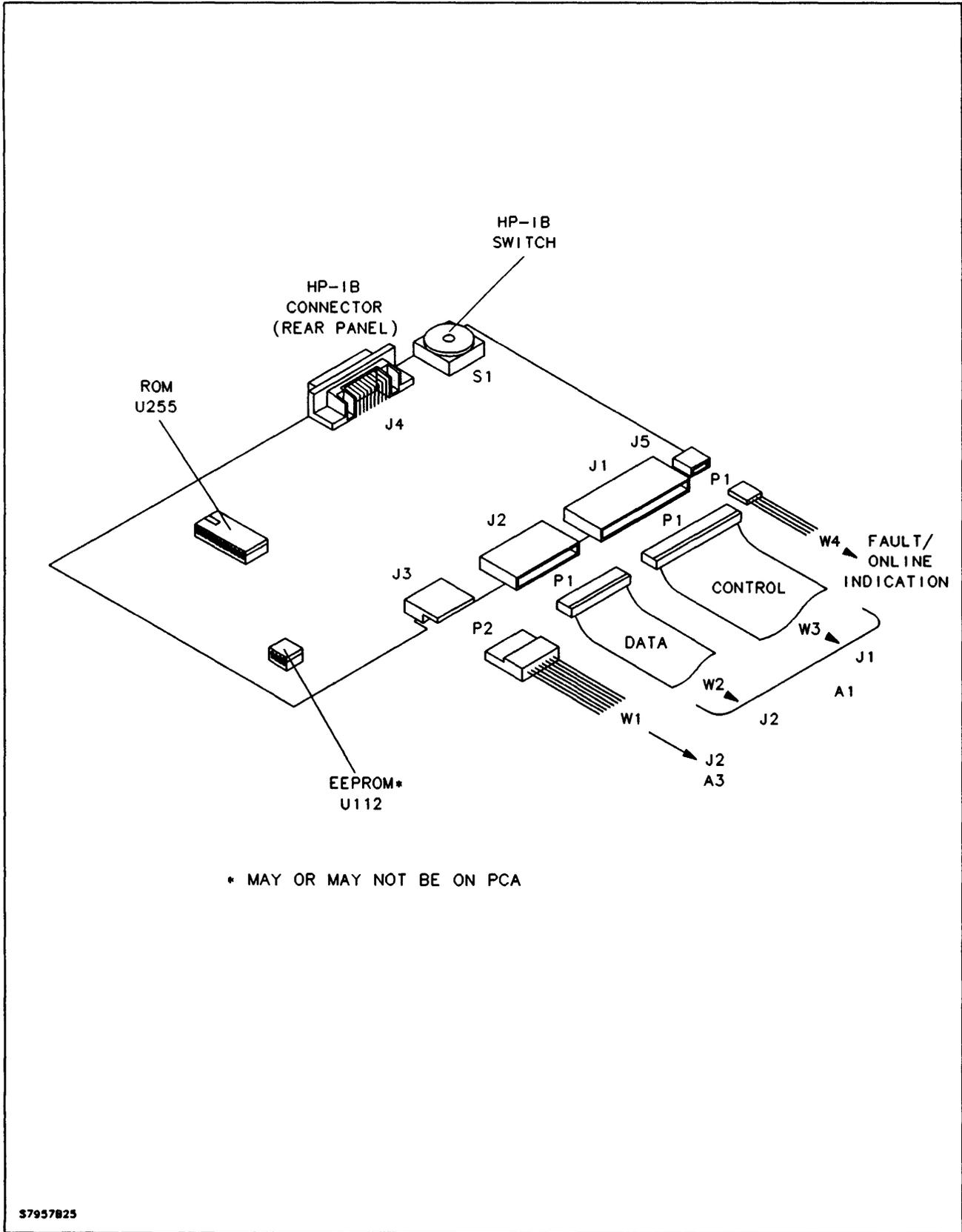
Figure 4-2. CS80/ESDI Controller (CEC) PCA-A2 Layout and Cable Connections
