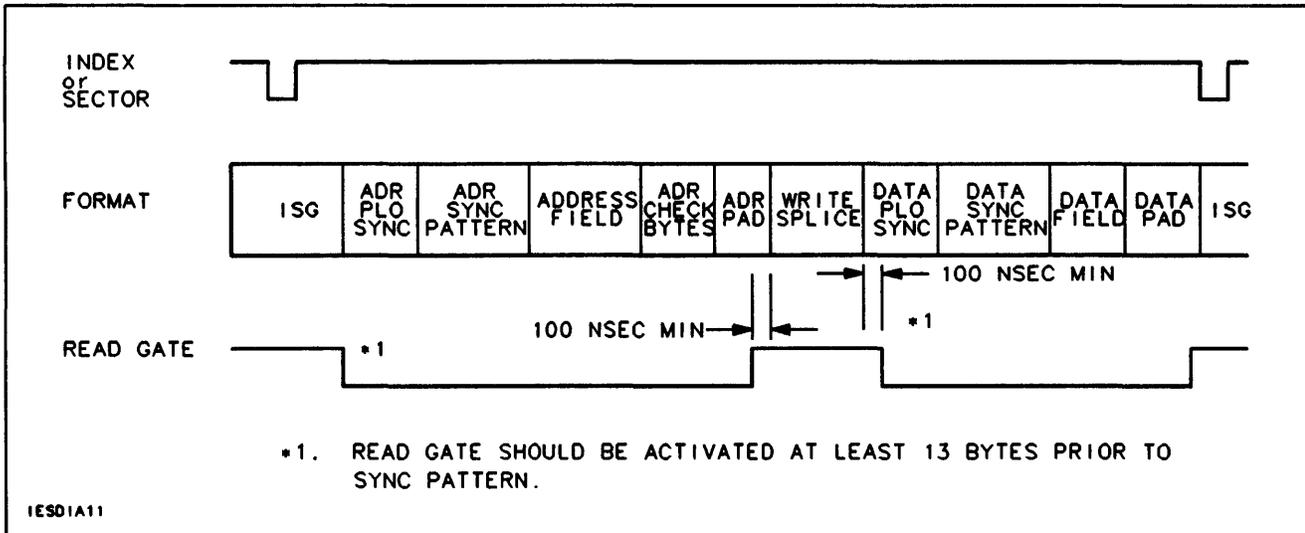
Figure 2-4. Read Gate Timing
