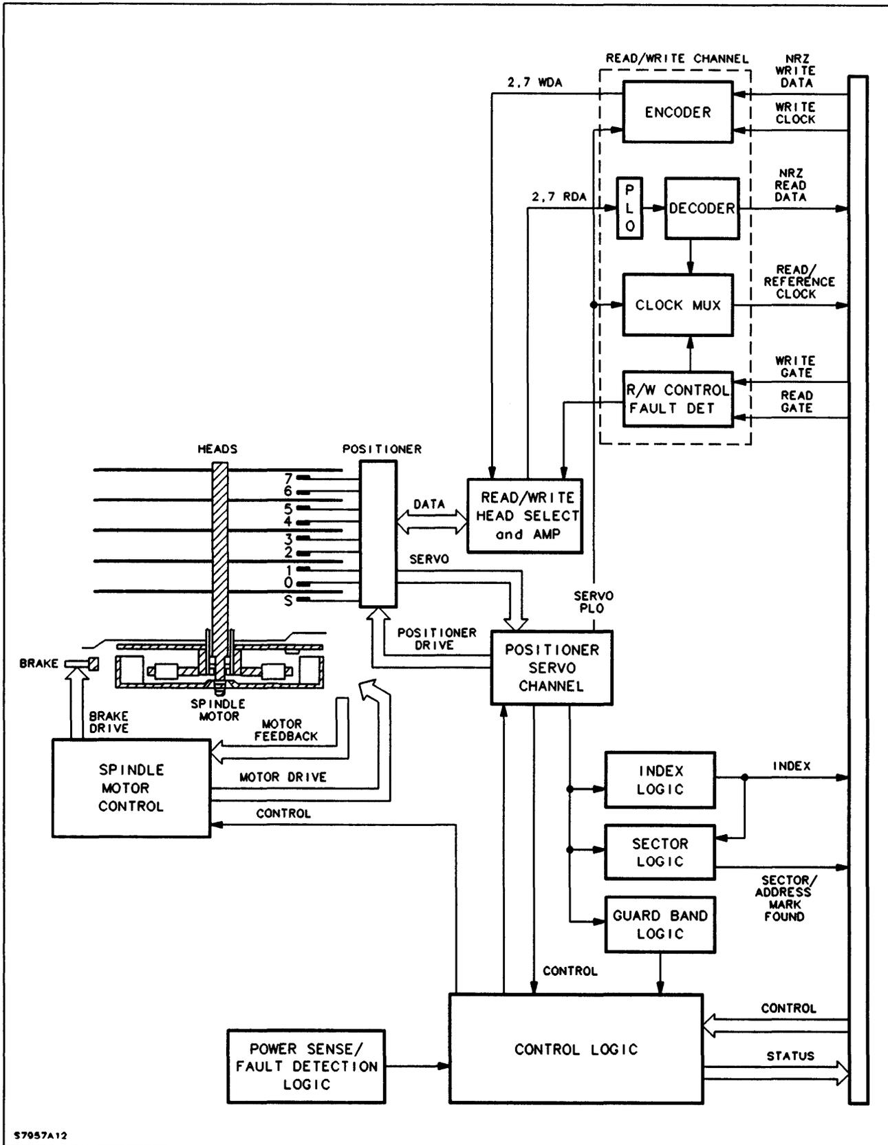
Figure 3-4. Disc Drive Assembly PCA-A1 Functional Elements
