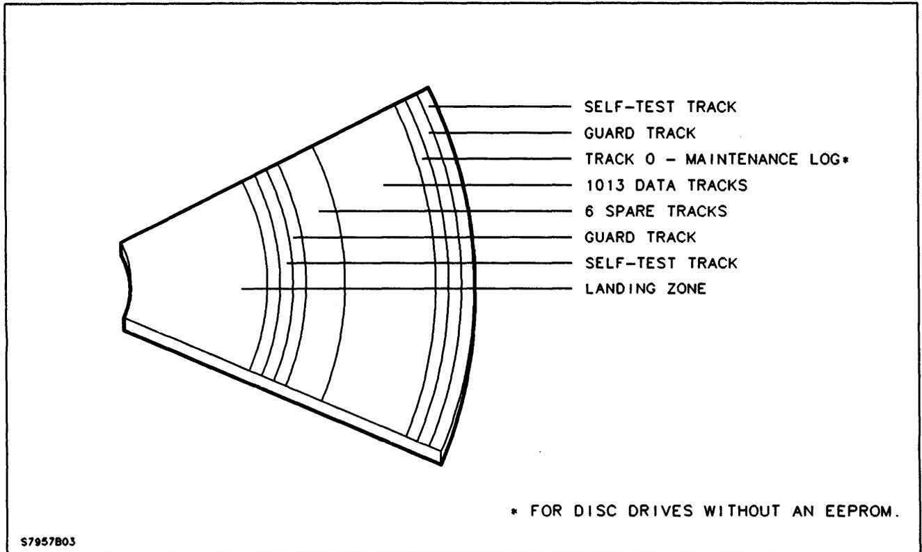
Figure 3-1. Disc Recording Format
