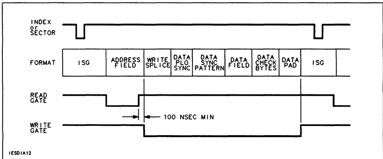
Figure 2-3. Write Gate Timing During Normal Write
