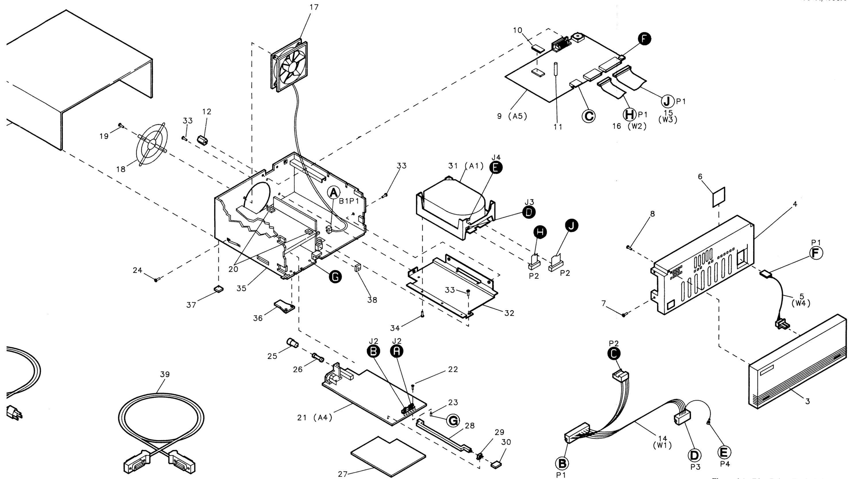
Figure 6-1. Disc Drive, Exploded View
