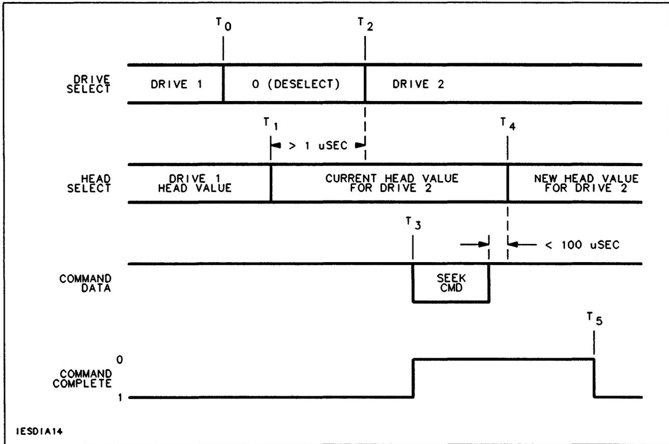
Figure 2-8. Recommended Drive/Head Selection Sequence
