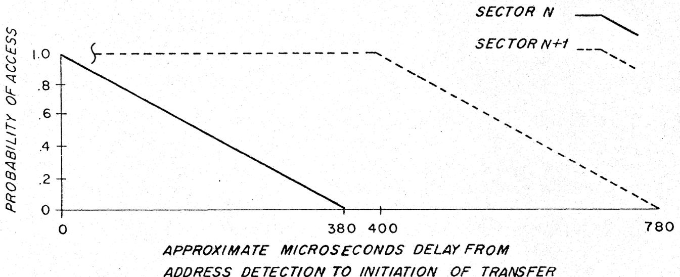
Figure 2. Sector Access Probability/Delay Time
