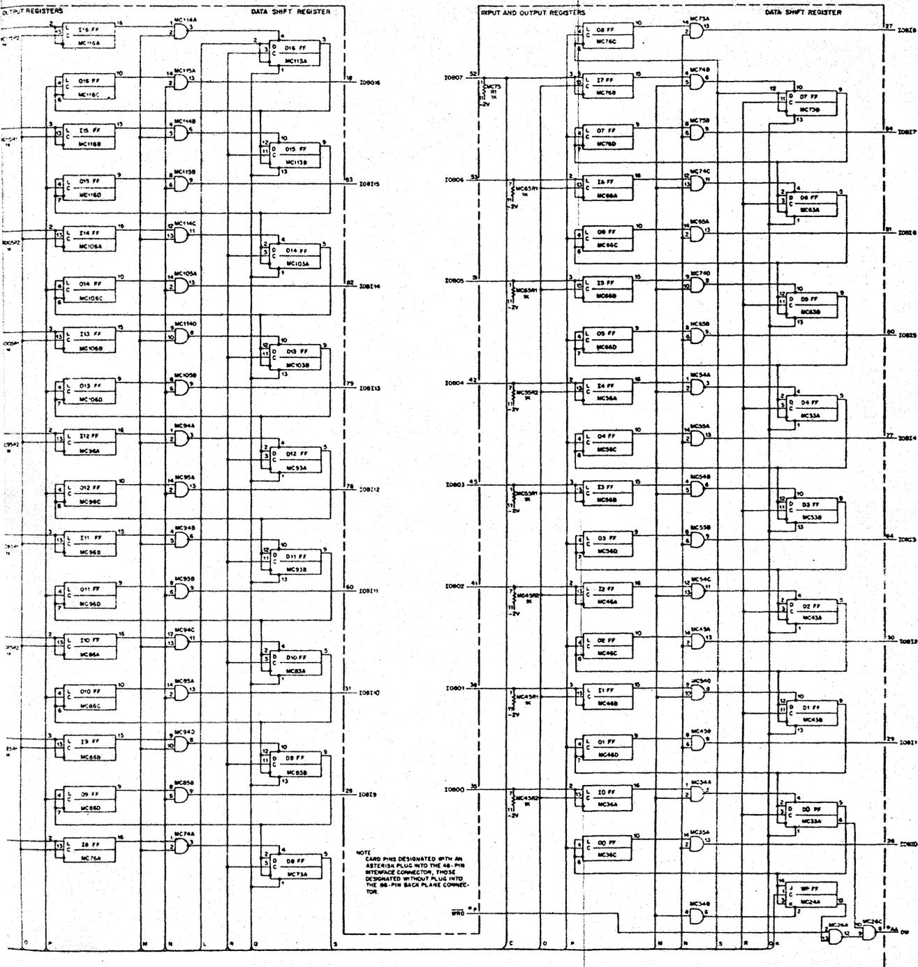
Figure 5-3. Data Channel Interface Card (12606-6001), Schematic Diagram
