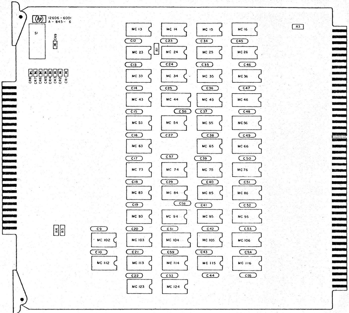
Figure 3. Data Channel Card (Part No. 12606-6001)
