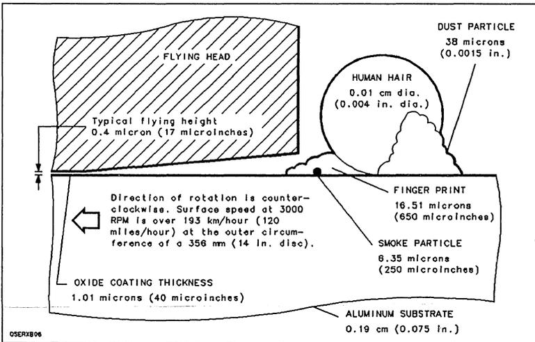
Figure 2-8. Contaminant Sizes Relative to Disc/Head Spacing
