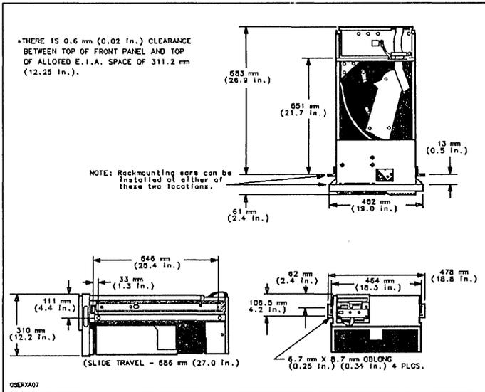
Figure A-1. HP 7911R/HP 7912R/HP 7914R Dimensions
