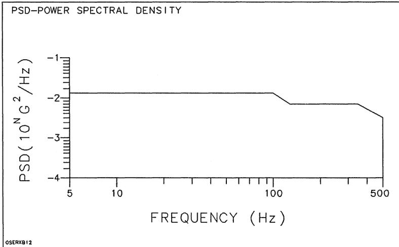
Figure 2-4. Random Vibration Profile 4: Nonoperating
