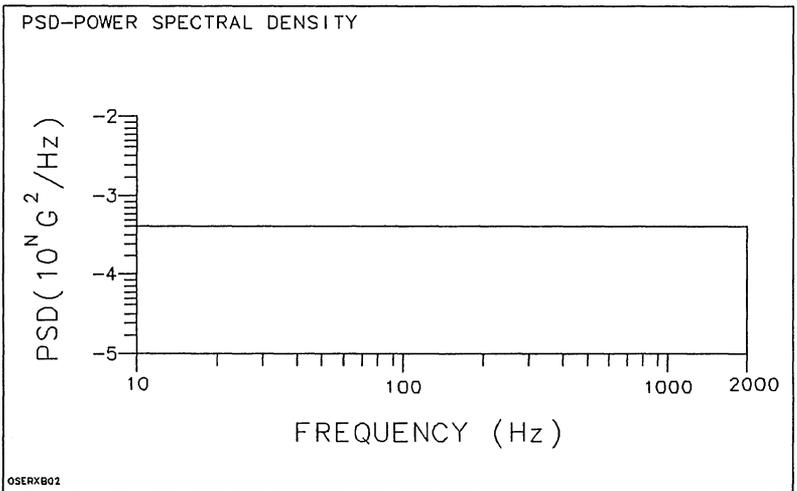
Figure 2-2. Random Vibration Profile 2: Nonoperating
