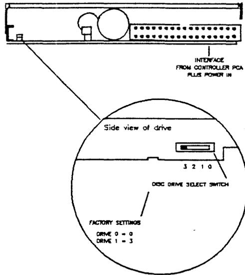
Figure 4-5. Disc Drive Select Switch (09123-69101).
