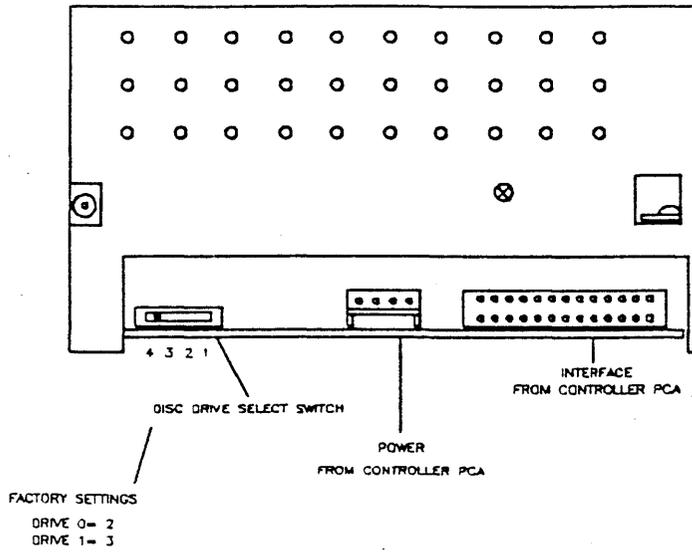
Figure 4-4. Disc Drive Select Switch(09114-69511).
