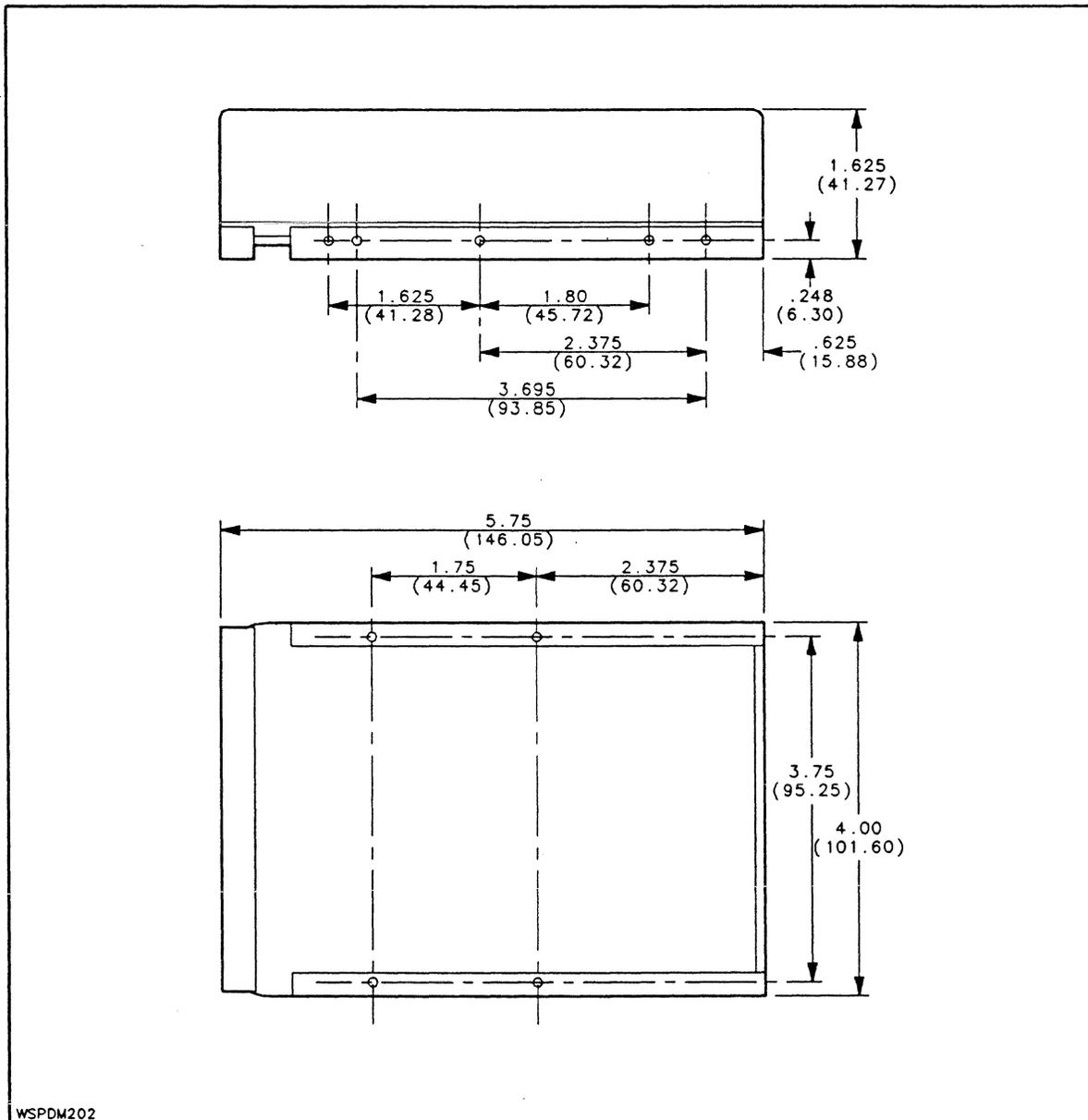
Figure 2-3. Connector Dimensions, Single-ended Unit.
