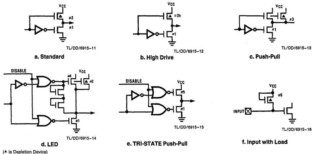
FIGURE 10. Input/Output Configurations
