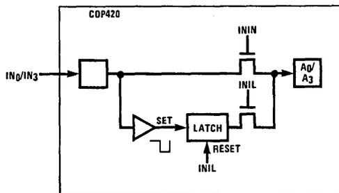
FIGURE 12. IN<sub>0</sub>/IN<sub>3</sub> Latches
