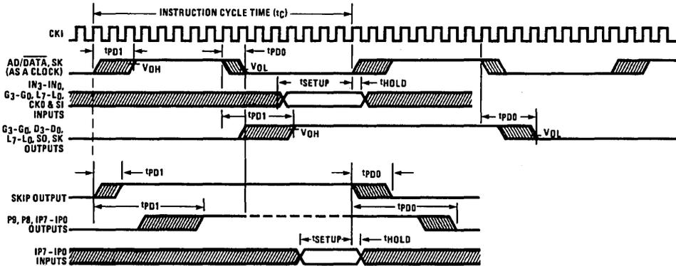
FIGURE 3a. Input/Output Timing Diagrams (Crystal ÷ 16 Mode)
