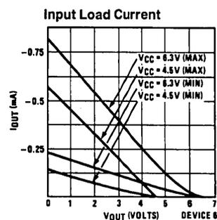
FIGURE 11. COP402/COP402M Input/Output Characteristics
