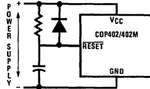
$$RC \geq 5 \times \text{Power Supply Rise Time}$$
