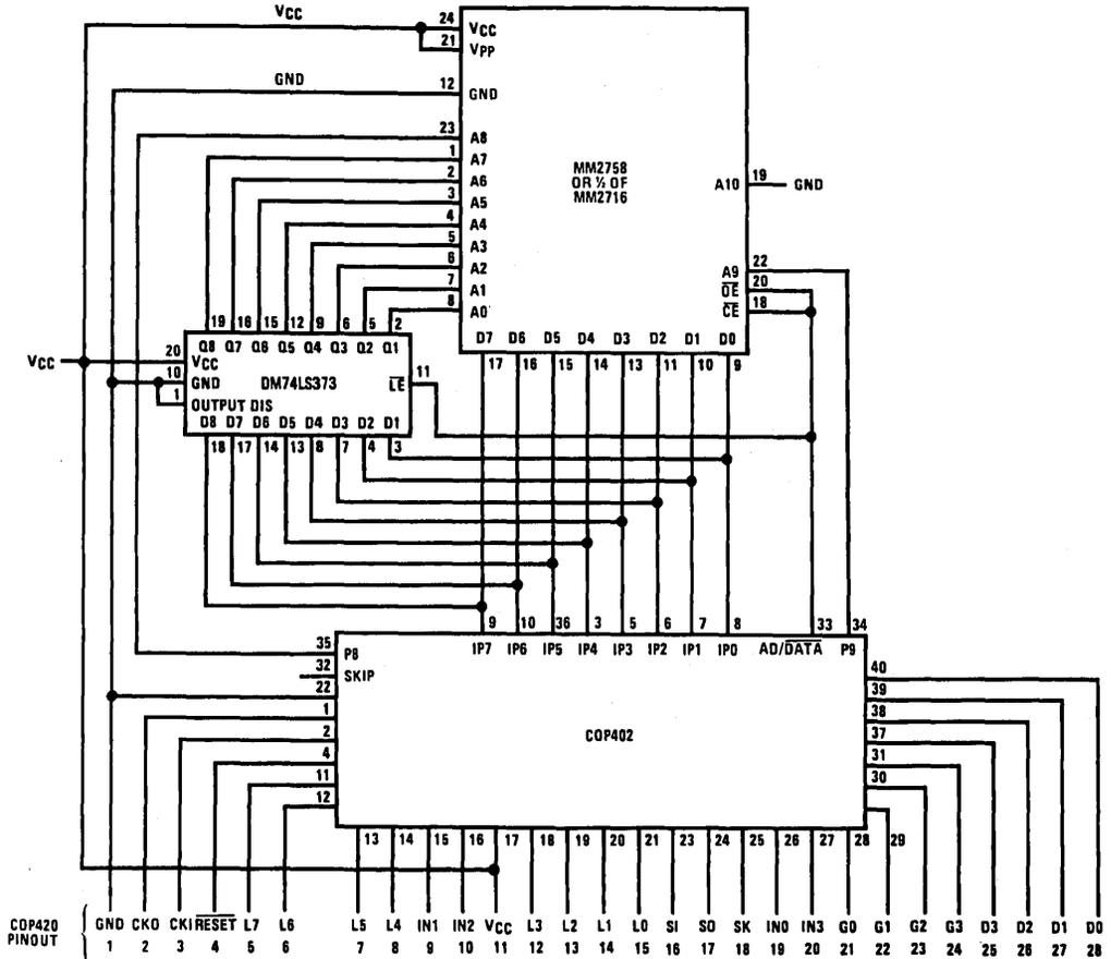
FIGURE 13. COP402 Used to Emulate a COP420
