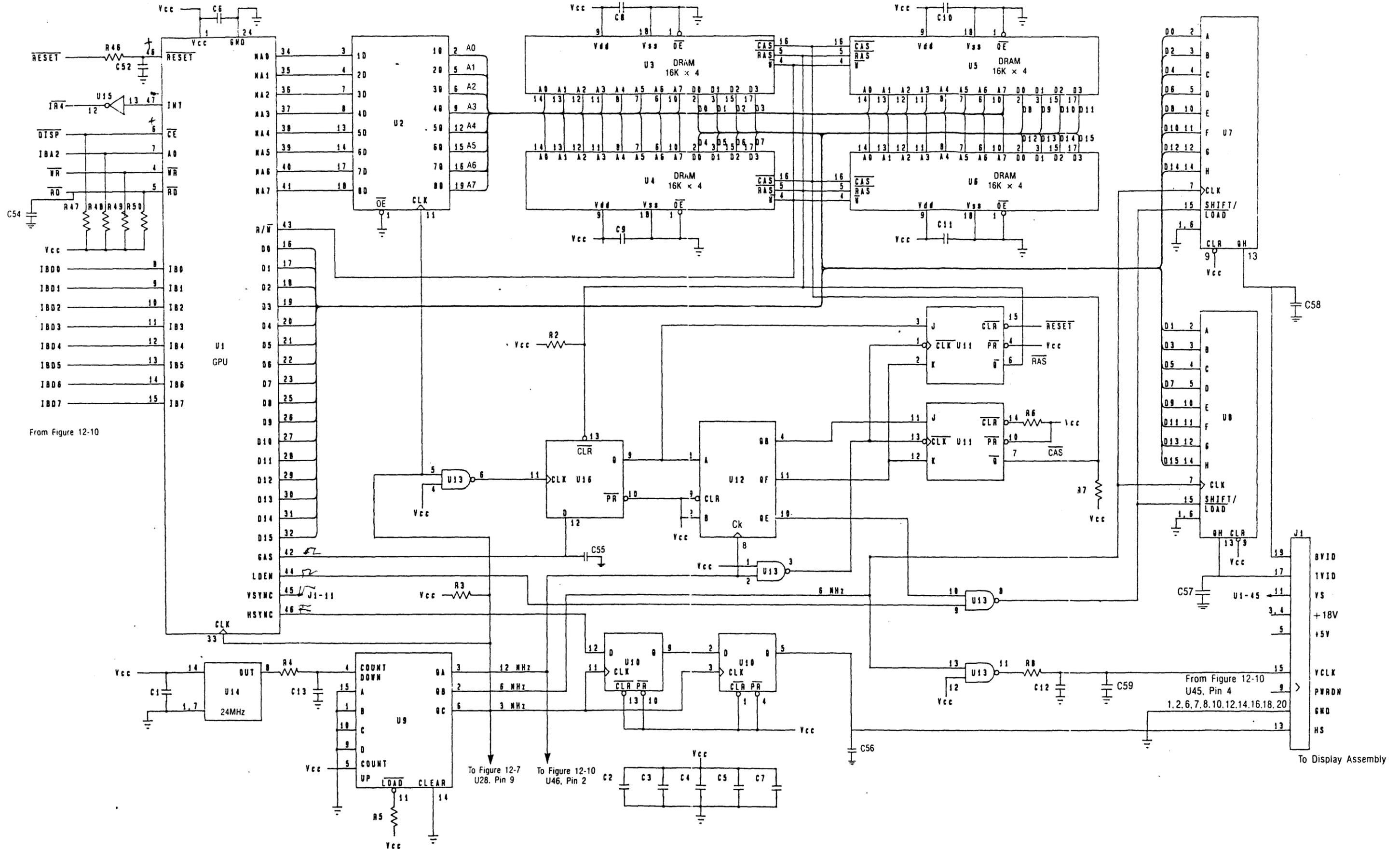
Figure 12-5. Logic B PCA—Display Control Schematic Diagram
