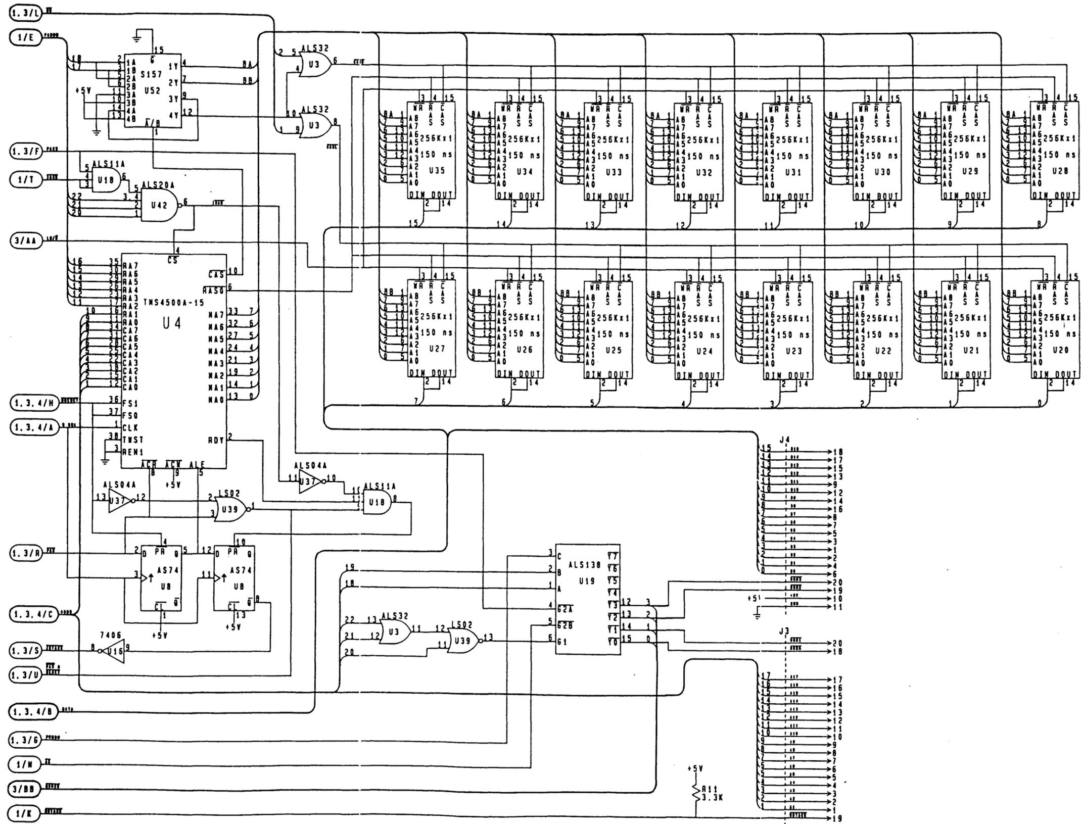
Figure 12-3. Logic A PCA—IDTACK, I/O, Logic B Interface Schematic Diagram
