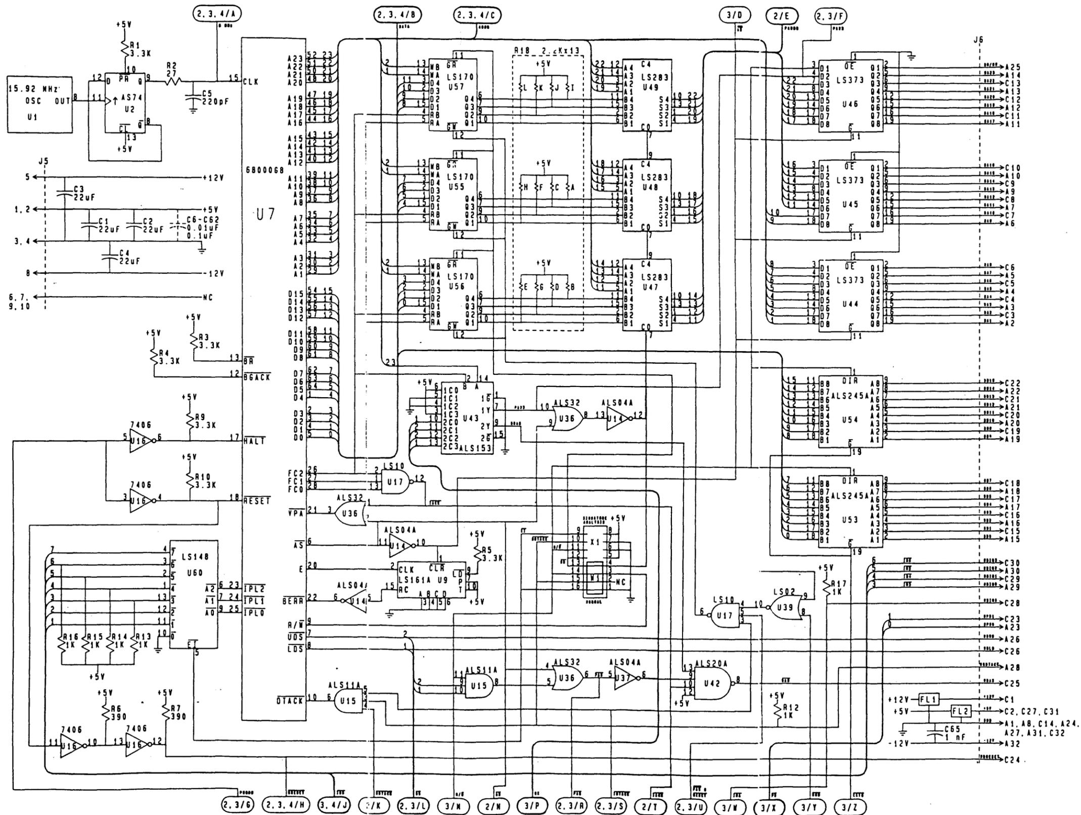
Figure 12-2. Logic A PCA—RAM, ROM Schematic Diagram
