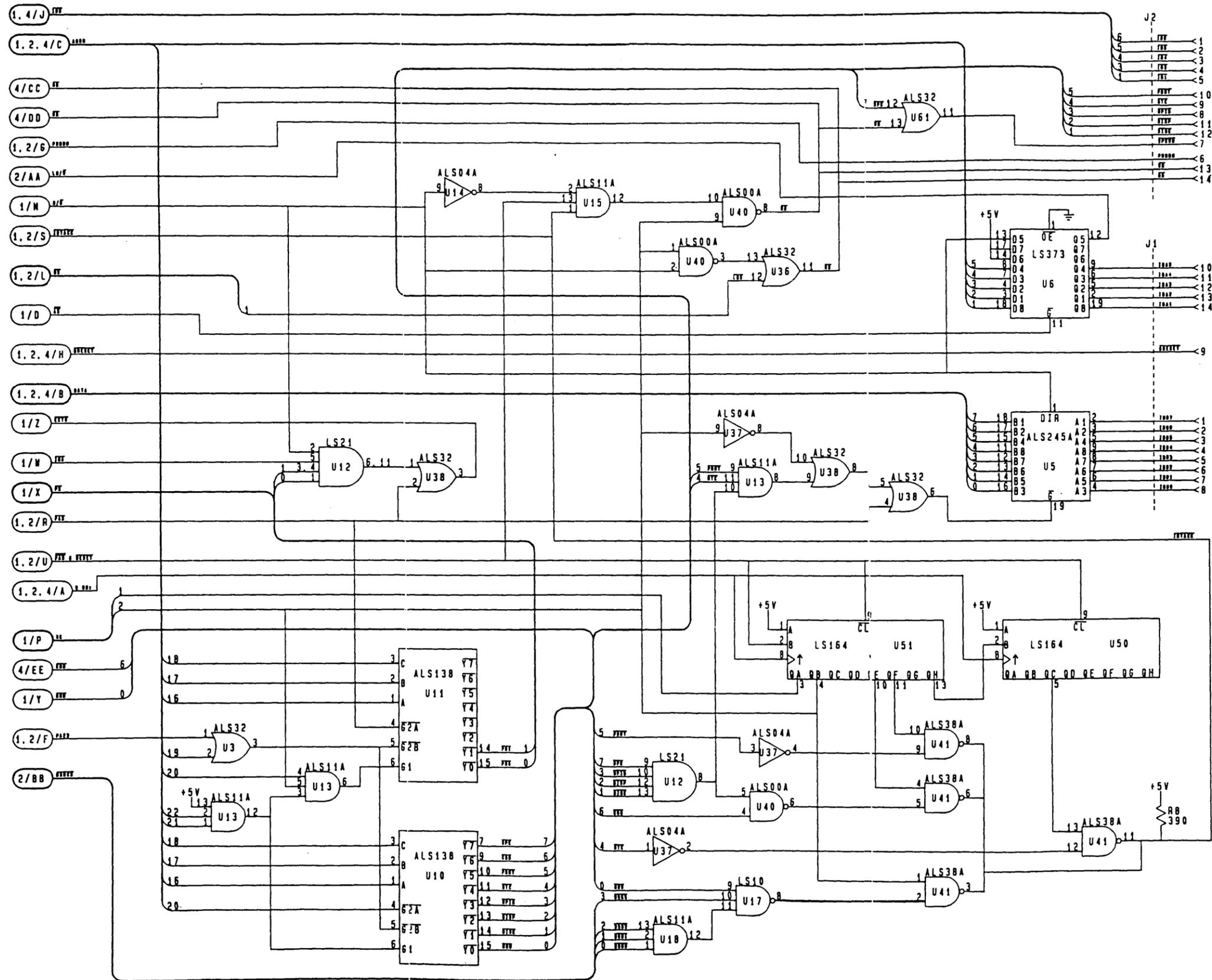
Figure 12-4. Logic A PCA—Keyboard Interface Schematic Diagram
