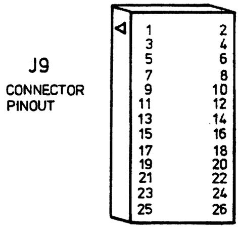
**Figure 8-8. Connector Pin Assignments**
