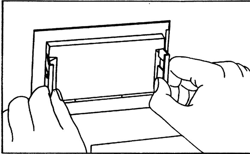
**Figure 6-41. Removing the System V ROM Assembly**
