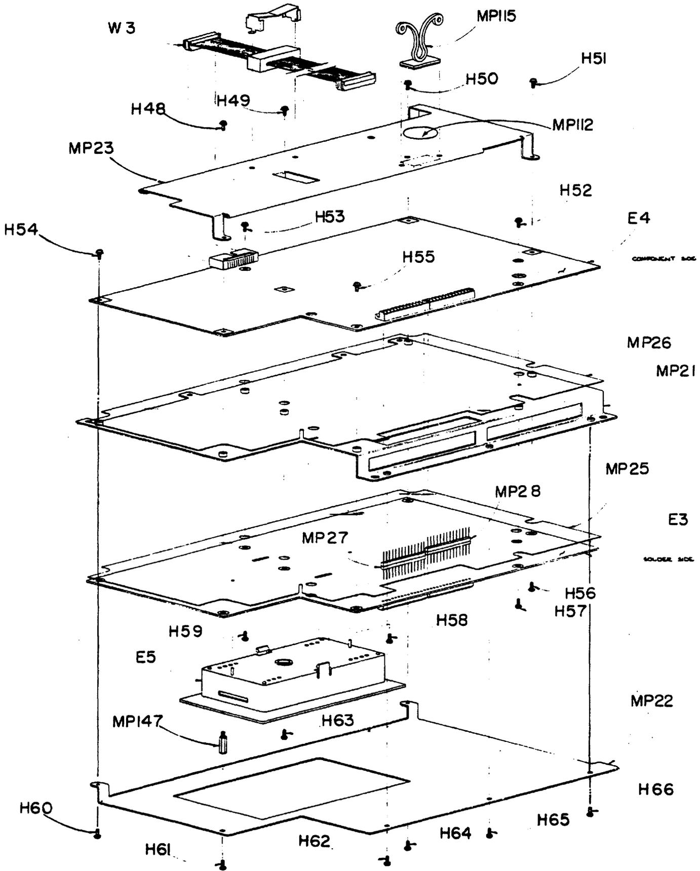
Figure 9-3. Logic Shield Assembly Exploded View
