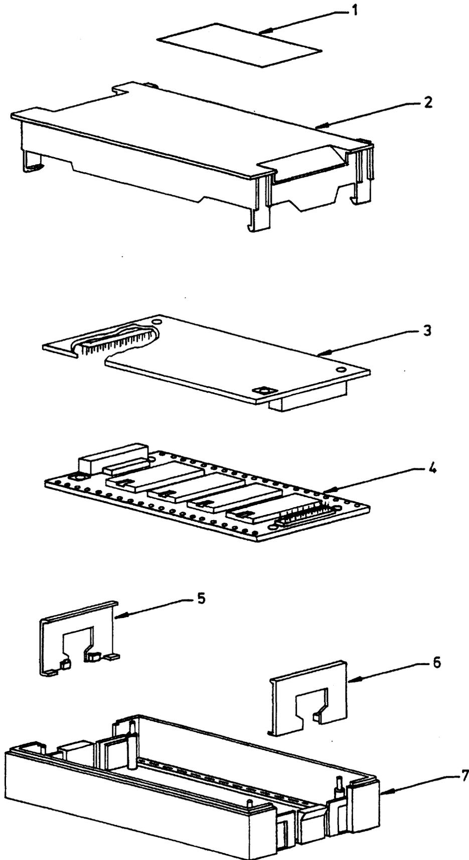
Figure 9-10. System V ROM Assembly Exploded View
