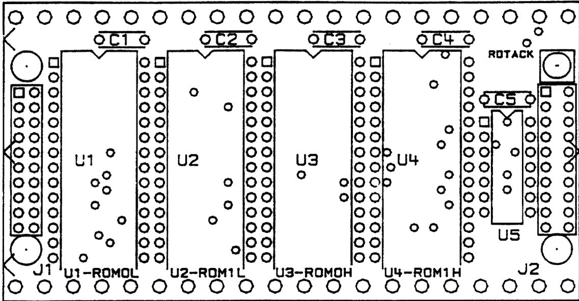
Figure 9-14. Operating System ROM PCA Component-Location Diagram
