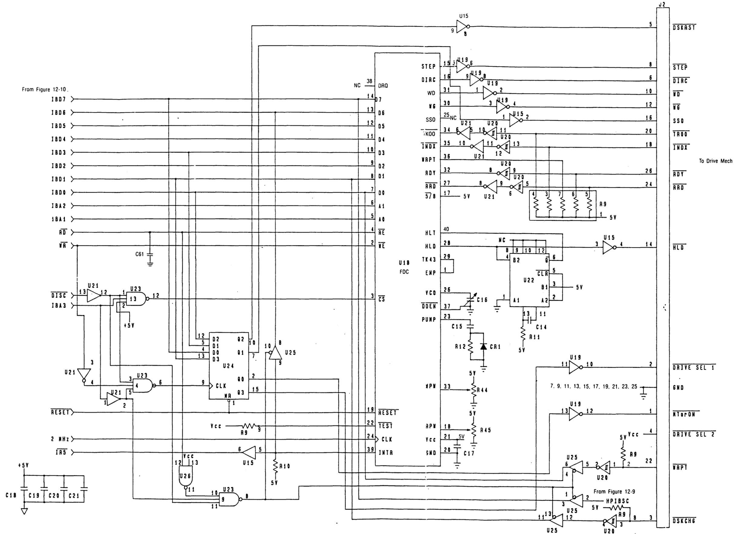
Figure 12-6. Logic B PCA—Disc Controller Schematic Diagram
