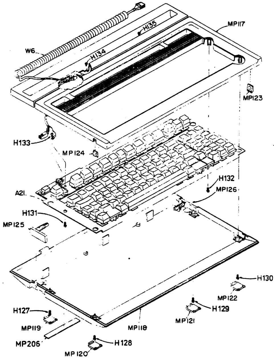
Figure 9-7. Keyboard Exploded View
