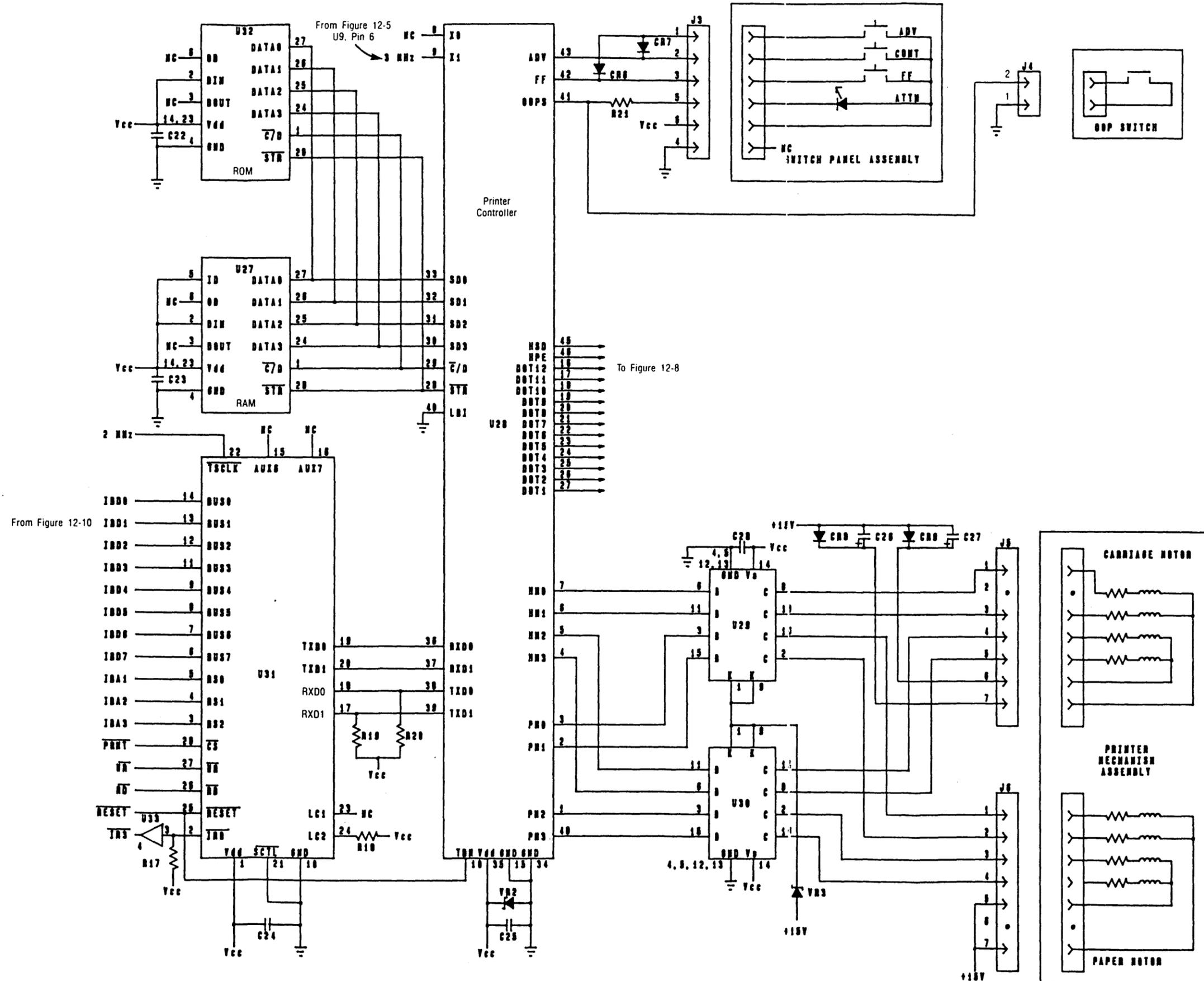
Figure 12-7. Logic B PCA—Printer Controller Schematic Diagram
