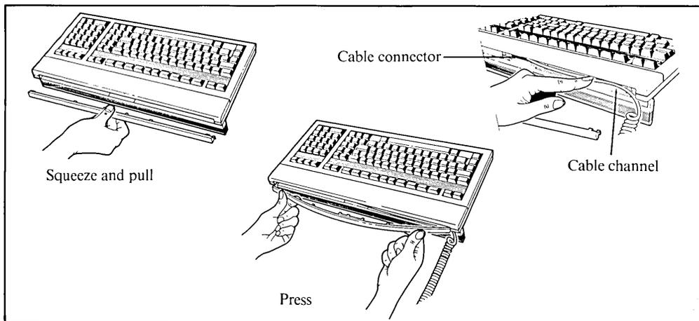
Figure 1-4. Keyboard Cable Cover
