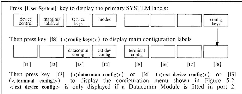
Figure 5-1. How To Display A Configuration Menu
