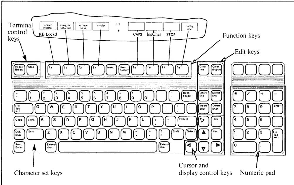
Figure 2-2. Function Keys And Screen Labels
