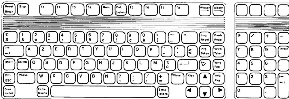
Figure 3-22. Flemish Keyboard (option 116) “VLAAMS”
