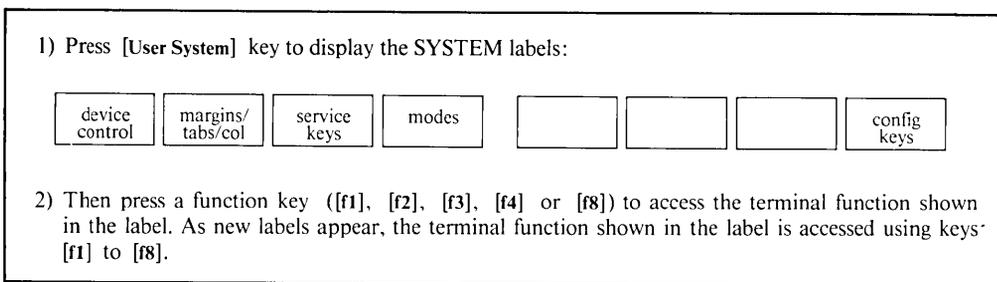
Figure 4-2. How To Use The Screen Labels
