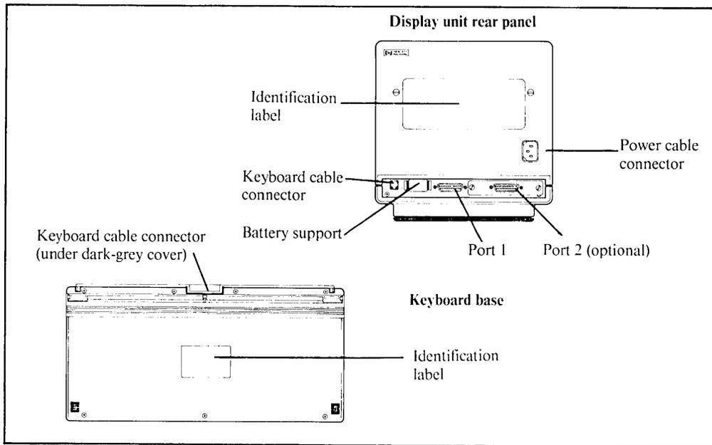
Figure 1-2. Rear Of Display Unit And Keyboard
