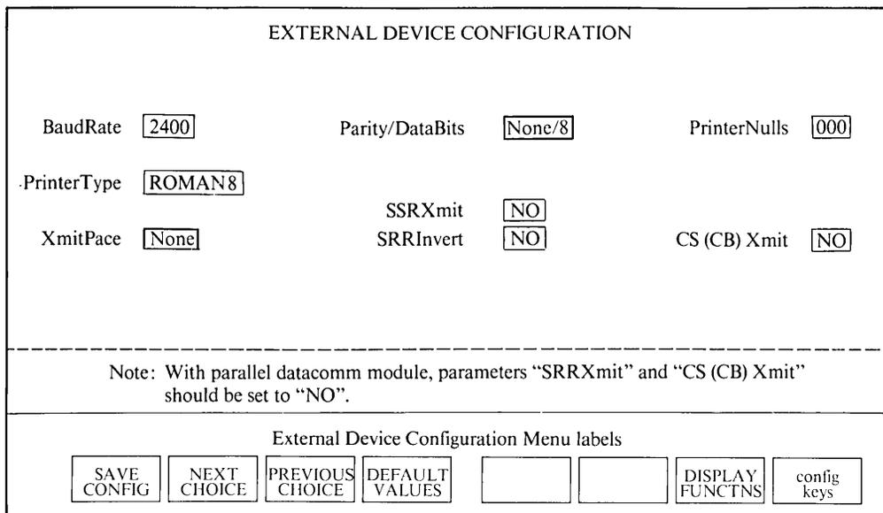
Figure 2-5. External Device Configuration Menu (Default Values)
