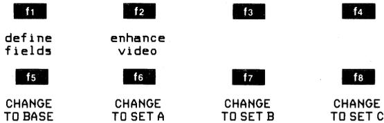
The **f1** and **f2** keys transfer you to the "define fields" and "enhance video" sets of function keys, respectively. The **f5** through **f8** keys activate the character sets currently specified by the @, A, B, and C fields (respectively) near the bottom of the Terminal Configuration menu. When you press one of the keys **f5** through **f8**, all characters from the current cursor
