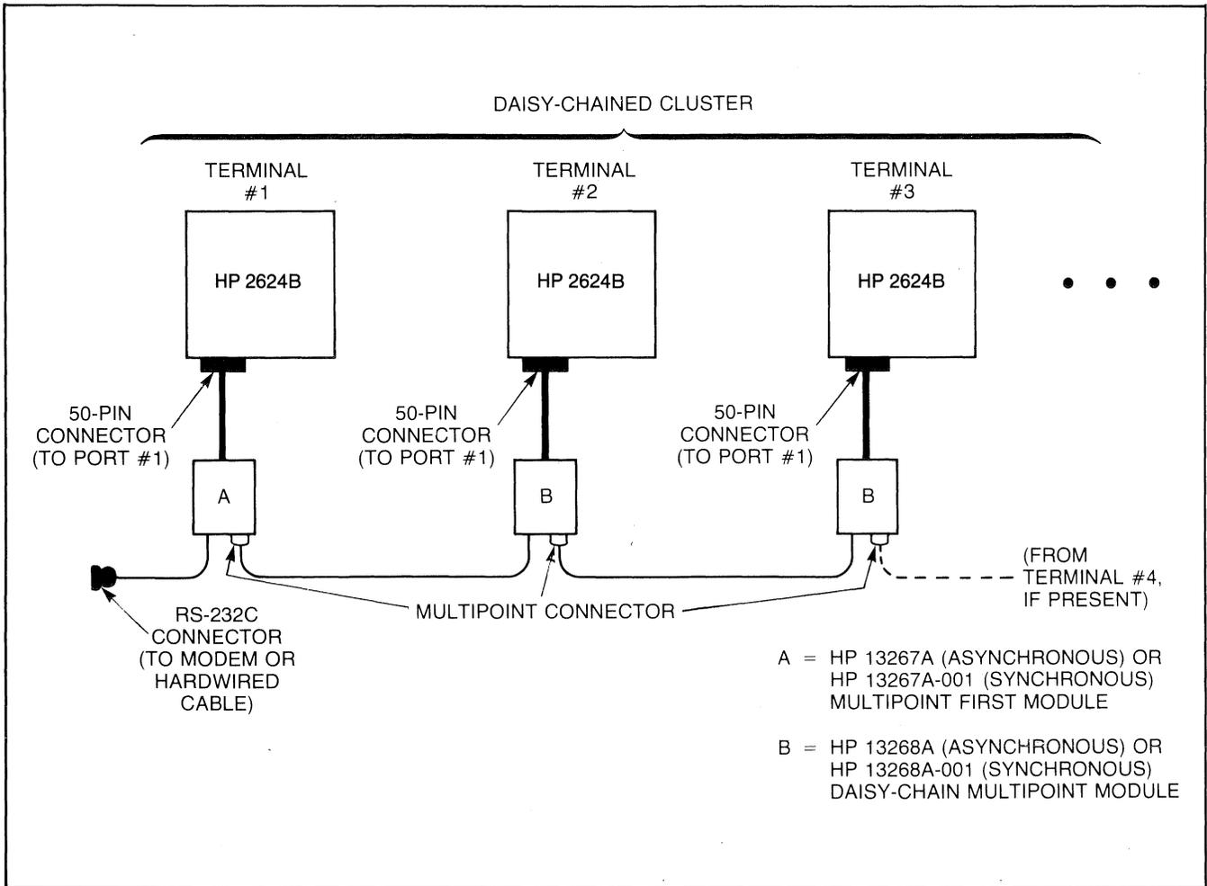
Figure 7-13. Port #1 Cabling (HP Multipoint Interfaces)
