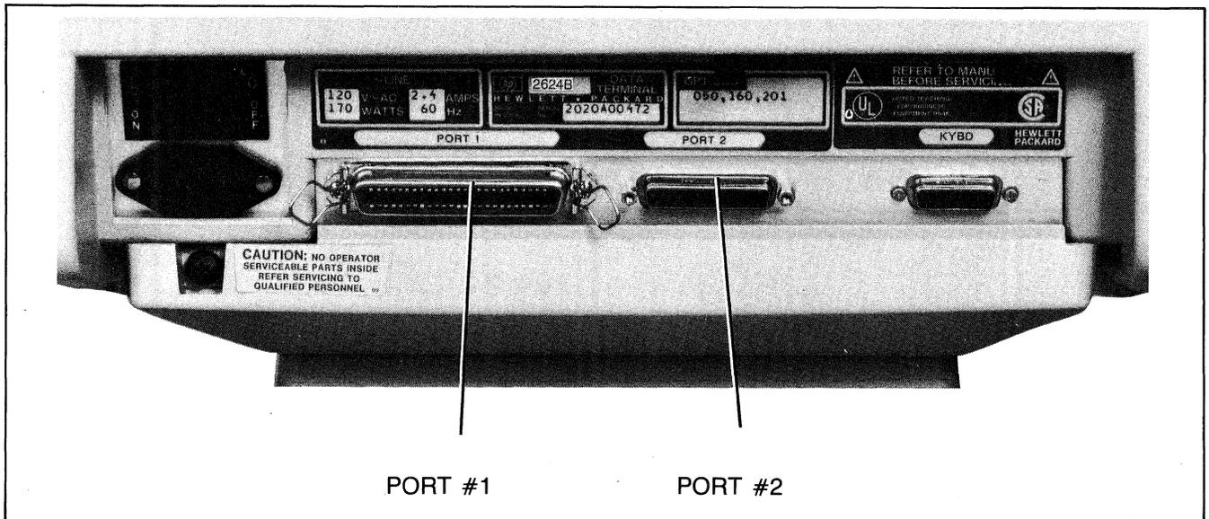
Figure 7-12. HP 2624B Display Terminal, Rear View
