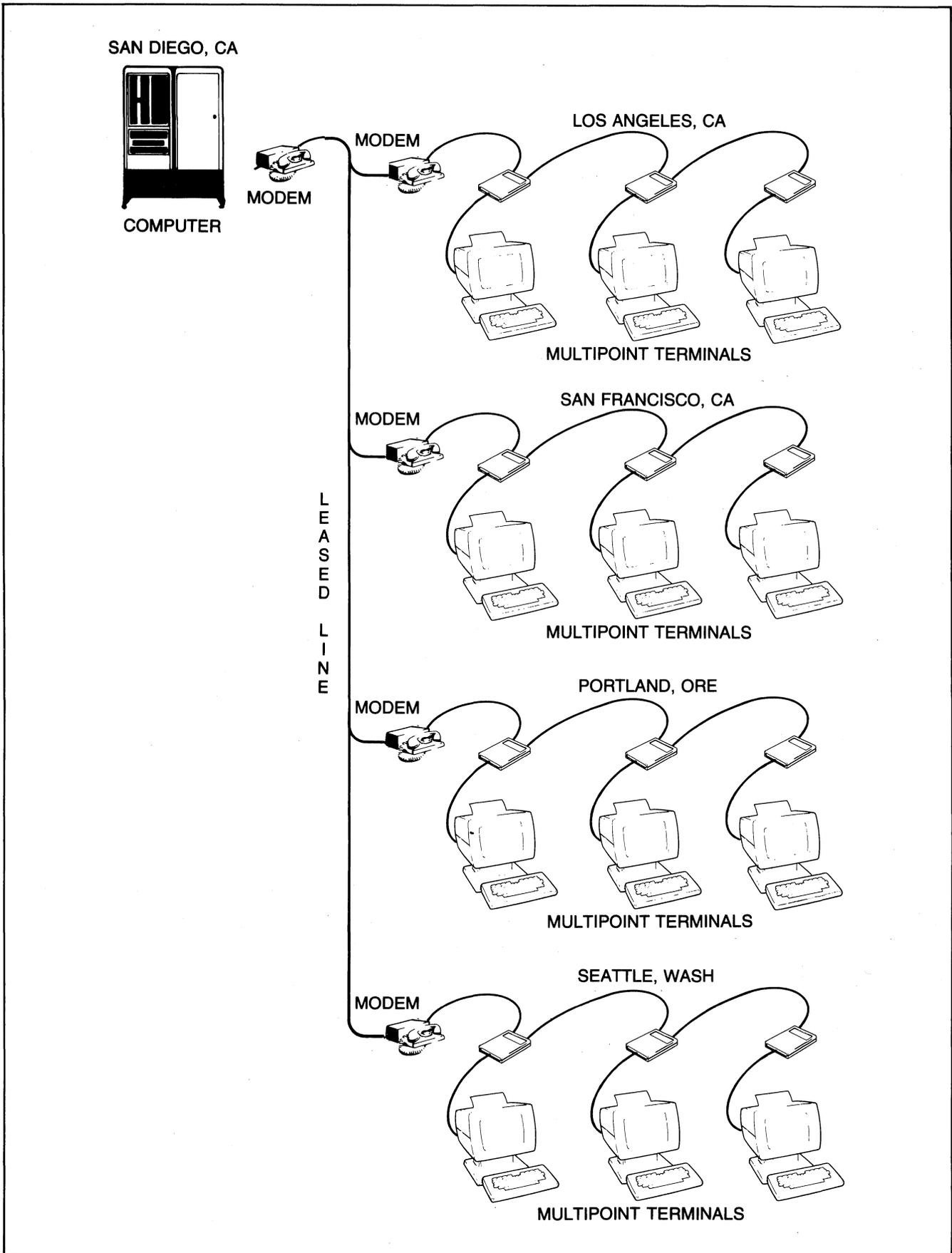
Figure 7-3. HP Multipoint Configuration (Leased Line, Multidrop)
