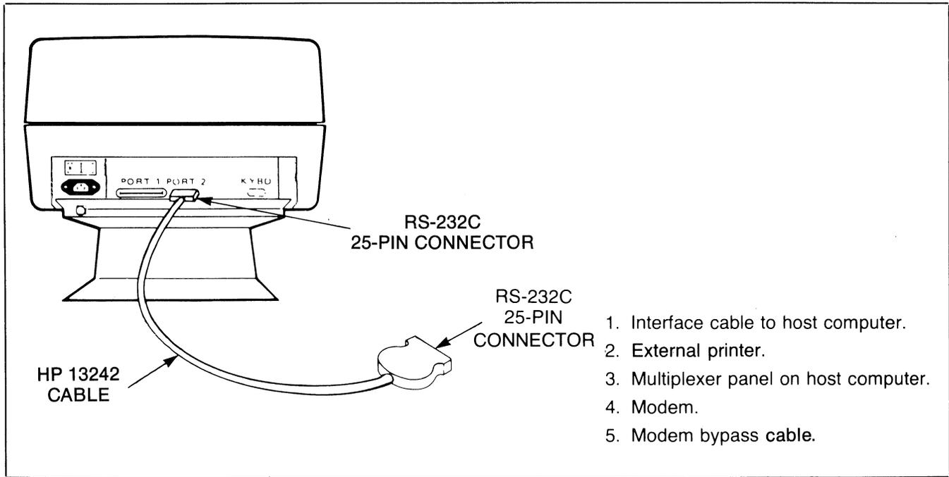
Figure 7-5. Port #2 Cabling (HP 13242 Cables)
