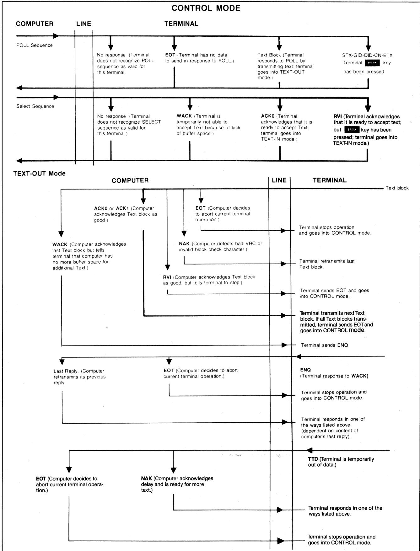
Figure 7-26. Operation of Block Protocol Control Characters
