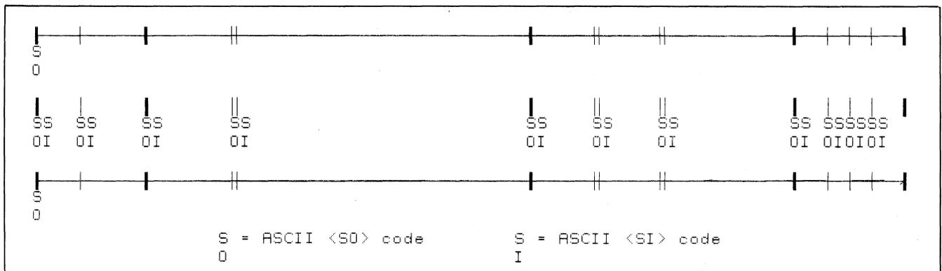
Figure 5-5. Use of Shift-In and Shift-Out Codes
