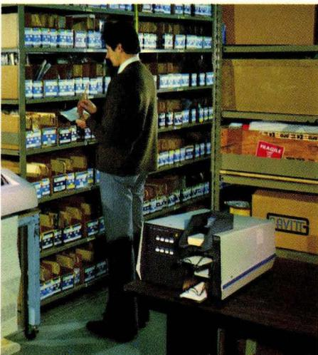
The 7260A is ideal for turn-around document applications where a line printer is used to print information on card stock. Additional information is manually marked on the cards and then using the 7260A reader, the information is transmitted to the host computer. Hewlett-Packard can provide documentation and support to the user for turn-around document design.
