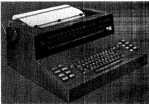
Figure 9. 1052 Printer-Keyboard
