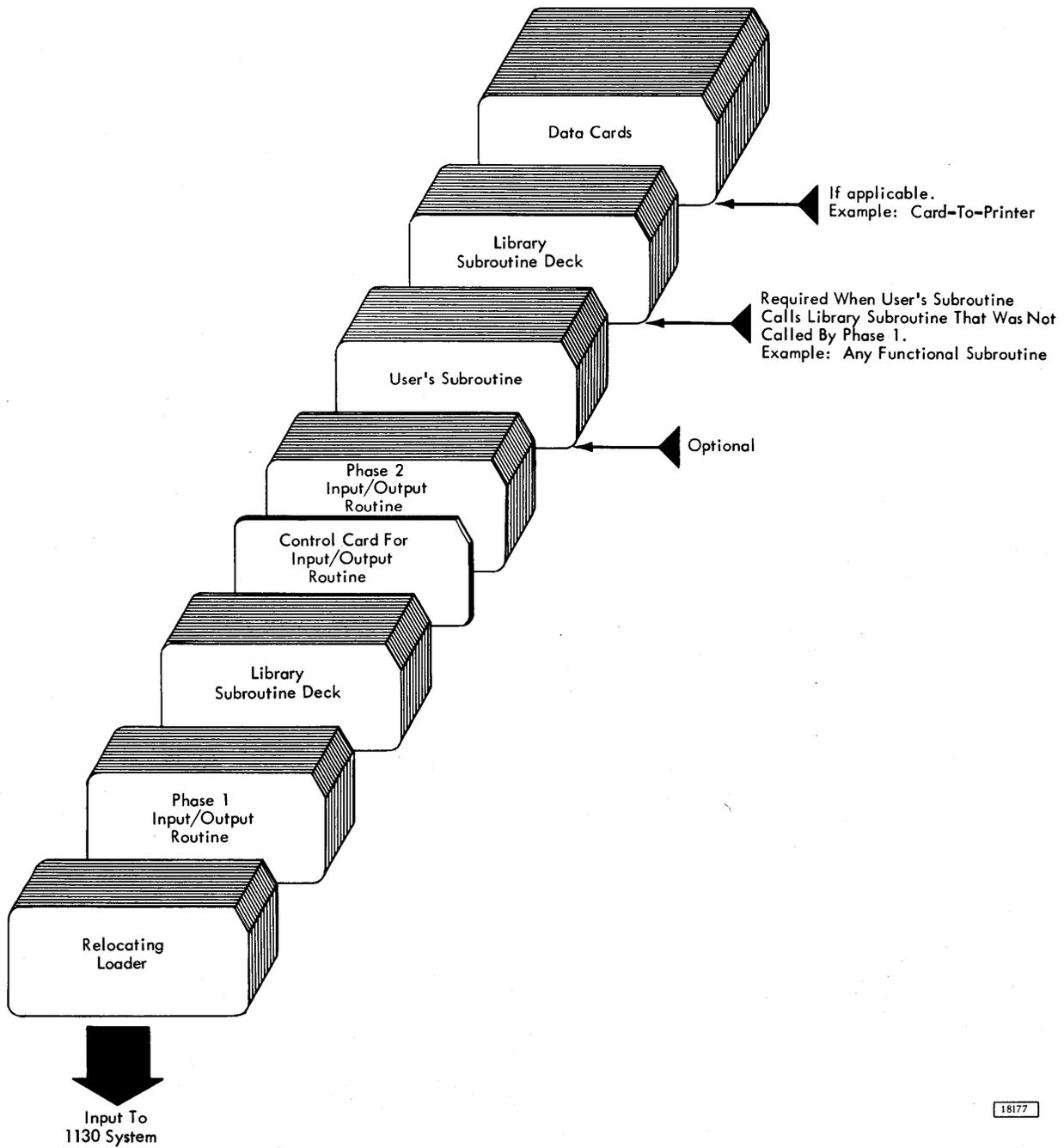
Figure 1. Stacked Input Arrangement for I/O Operations
