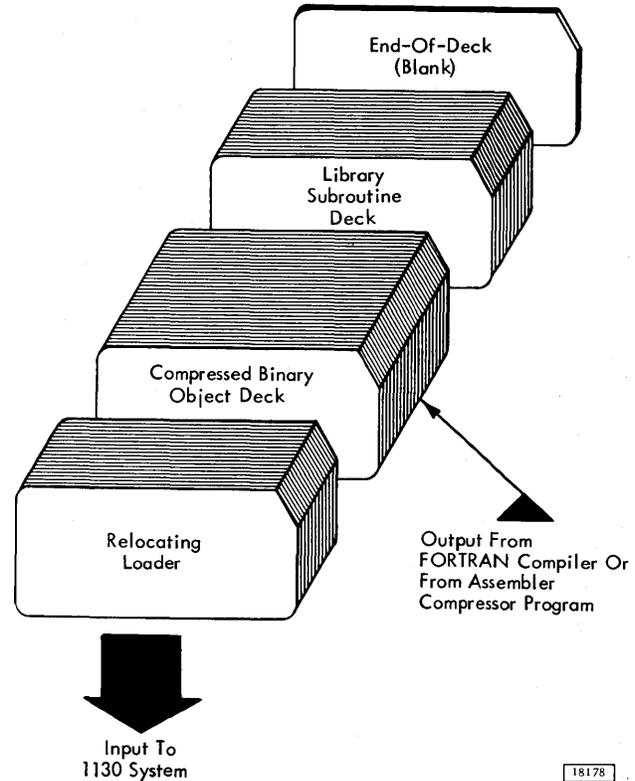
Figure 2. Stacked Input to Load a Relocatable Program
