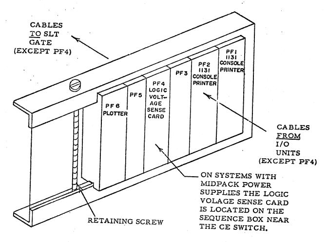
NOTE: POSITIONS PF1 AND 2 ARE BASIC AND PROVIDE CONNECTIONS TO THE 1131 CONSOLE PRINTER. PF4 IS BASIC AND HOLDS THE LOGIC VOLTAGE SENSE CARD. POSITIONS PF3, 5 AND 6 ARE FEATURE CONNECTORS.
