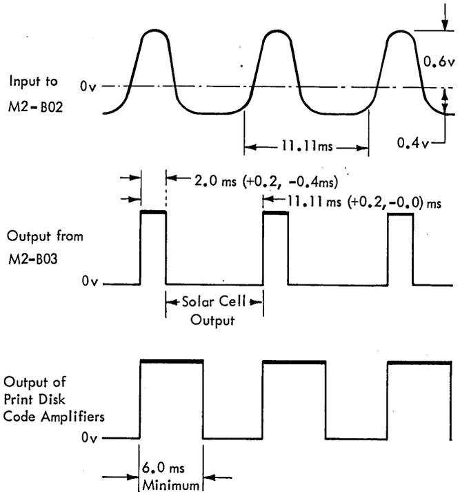
Note: Shown with print disk turning at approximately 112.5 rpm which results in a print clutch shaft speed of 300 rpm.
