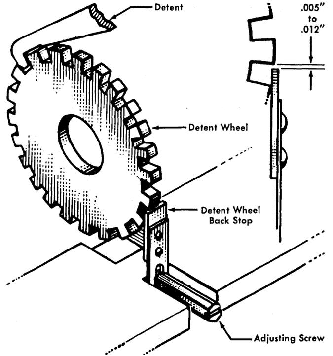
Figure 4-24. Detent Wheel Backstop
