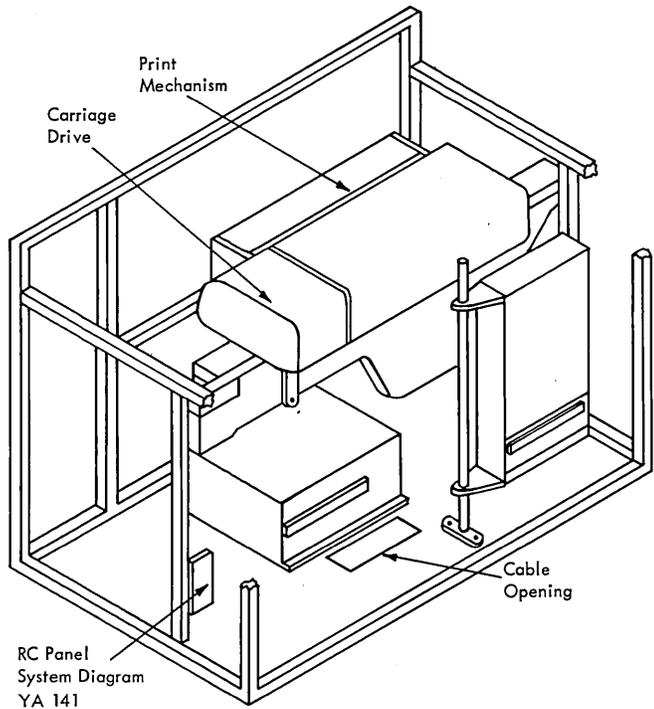
Figure 6-2. 1132 Printer - Rear View
