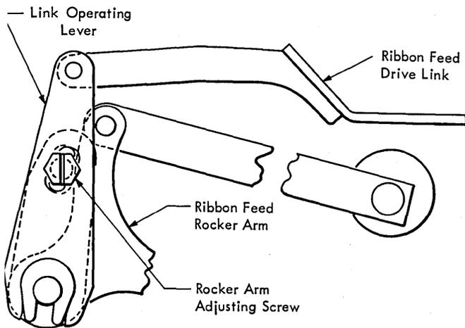
Figure 4-10. Ribbon Feed Stroke
