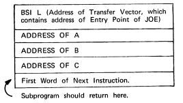
When a SUBROUTINE subprogram CALL is used, results of the computations within the subprogram will be returned by means of the arguments. The Assembler coded SUBROUTINE subprogram must return control to the calling program at the next location following the last argument in the list.
