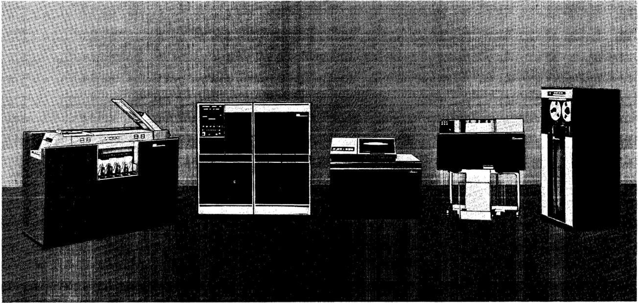
Figure 29. IBM 1401, Using IBM 1311 Disk Storage
