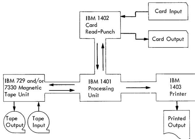
Figure 24. Data Flow (Tape System)
