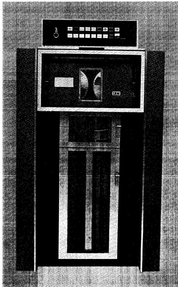
Figure 50. IBM 7340 Hypertape Drive Model 2
