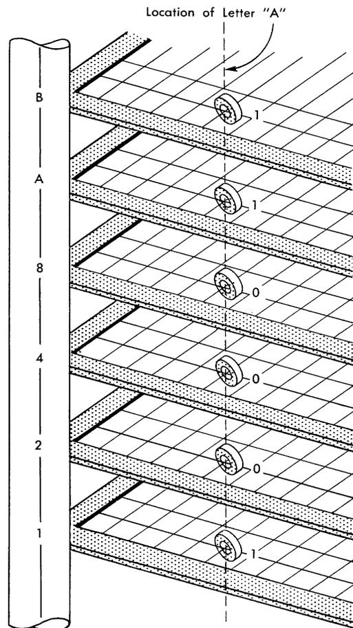
Figure 4. The Letter A Represented in Magnetic-Core Storage
