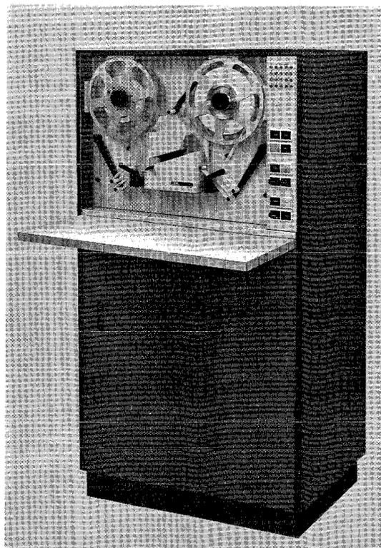
Figure 42. IBM 1012 Tape Punch
