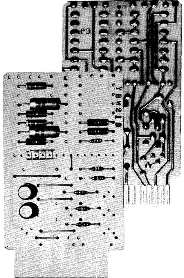
Figure 6. Transistor Cards
