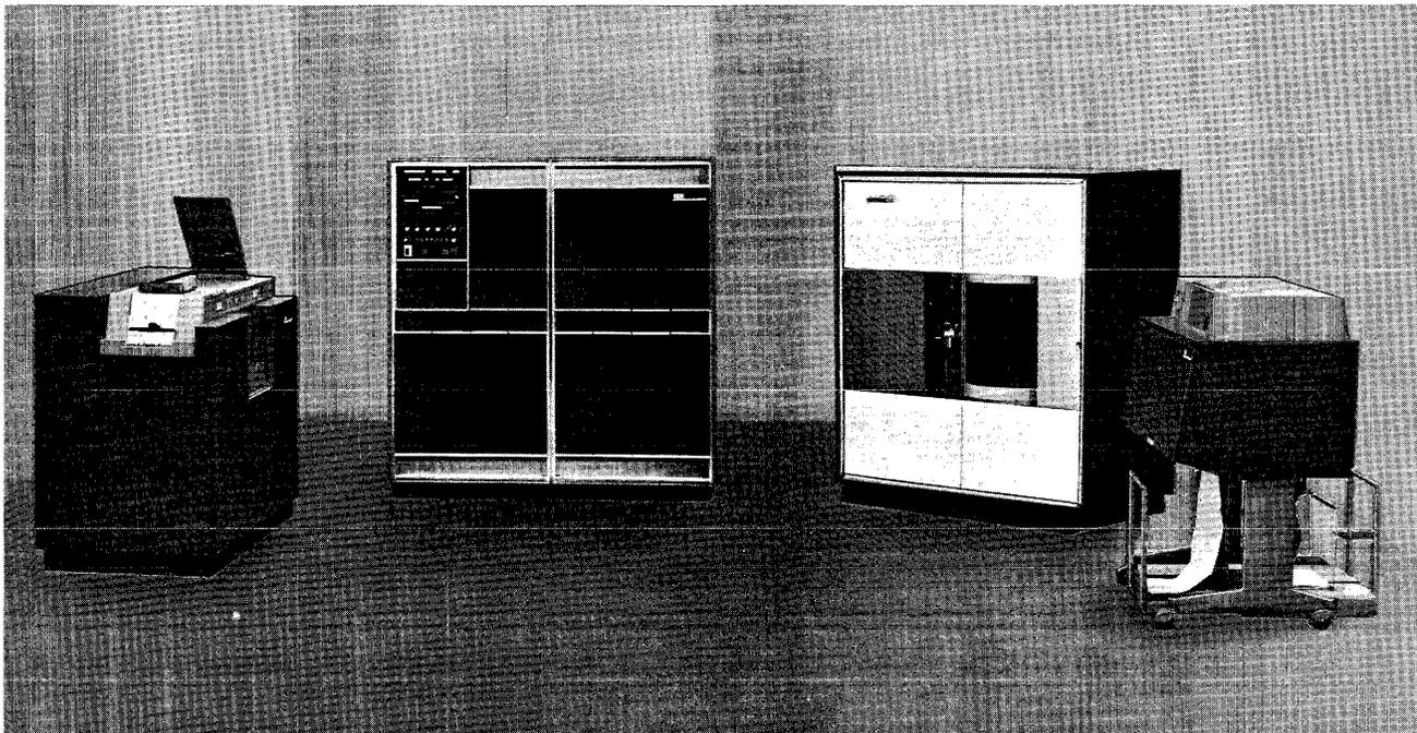
Figure 28. IBM 1401, Using IBM 1405 Disk Storage
