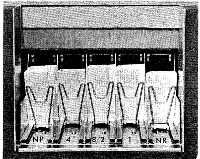
Figure 11. Radial Stackers
