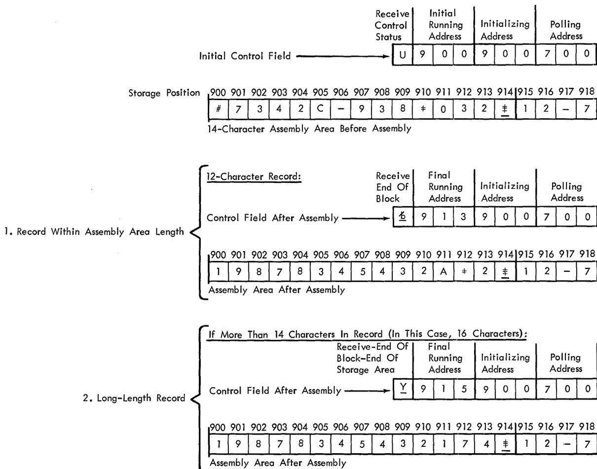
Figure 10. Scan Operation and Control Field During Assembly
