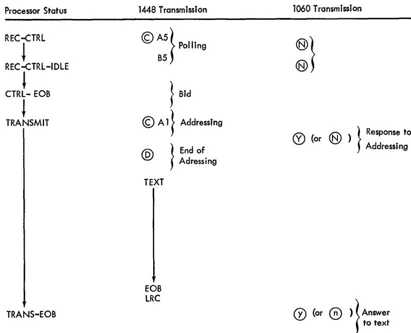
Figure 18. General Multipoint, Half-Duplex Operation (Processing Unit-1448 to 1060)
