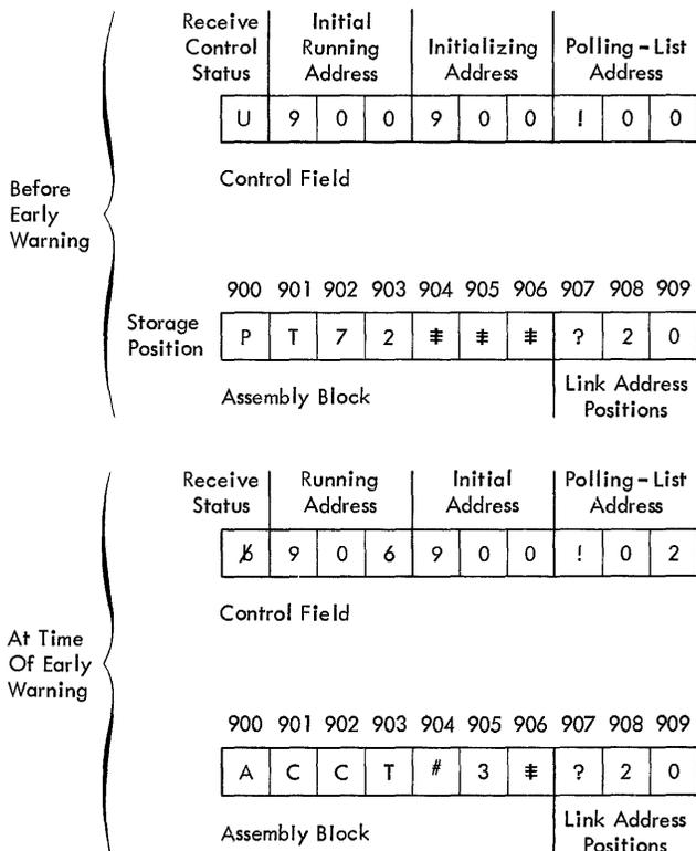
Figure 14. Control Field and Assembly Block During Early-Warning
