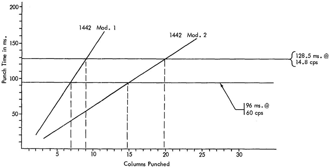
Figure 24. Punch Time vs. Columns Punched (1442)
