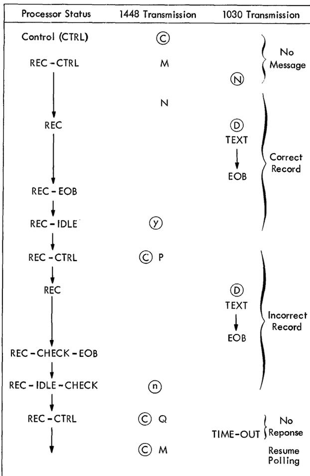
Figure 17. General Multipoint, Half-Duplex Operation (1030 to Processing Unit-1448)
