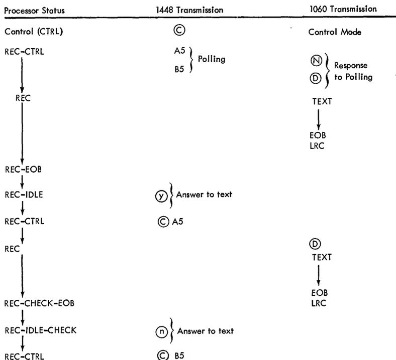
Figure 16. General Multipoint, Half-Duplex Operation (1060 to Processing Unit-1448)
