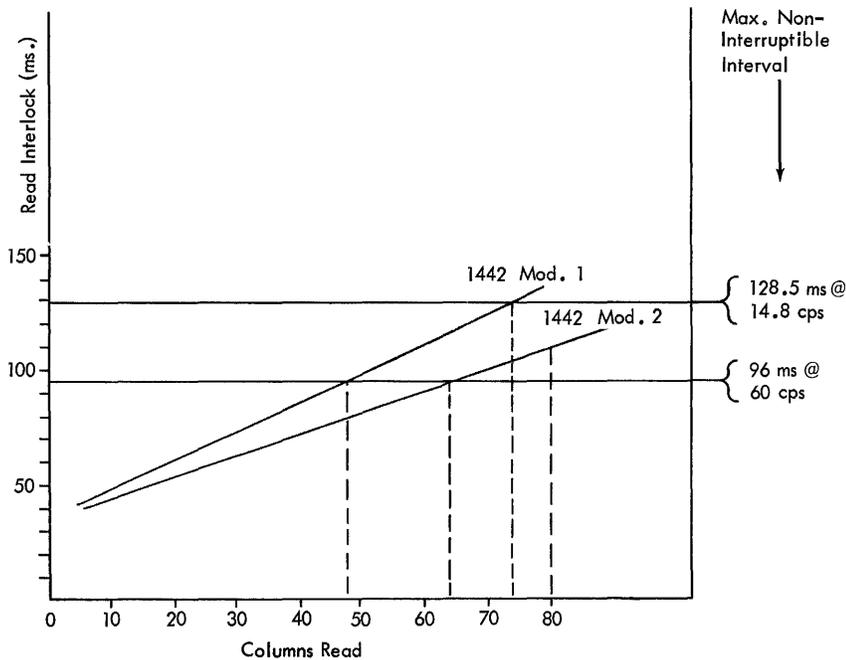
Figure 23. Read Interlock Time vs. Columns Read (1442)
