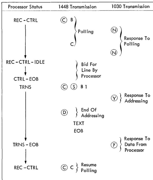
Figure 19. General Multipoint, Half-Duplex Operation (Processing Unit-1448 to 1030)
