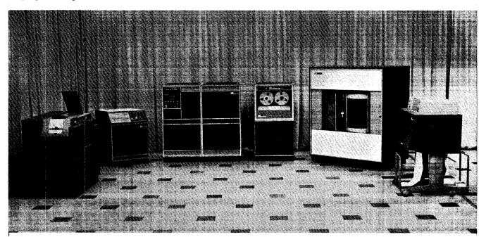
Figure H-1. The IBM 1401 or 1460 with 1009 Terminal
