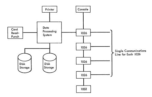
Figure H-96. IBM 1026 Transmission Control Unit
