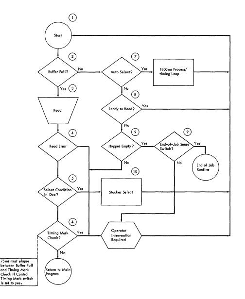
Figure H-98. IBM 1231 Continuous Feed Routine
