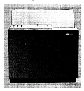
Figure H-97. IBM 1231 Optical Mark Page Reader
