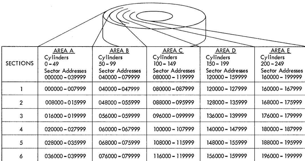
NOTE: Numbers shown above are the sector addresses of the lowest - and highest - numbered sector addresses in each section of each area.
