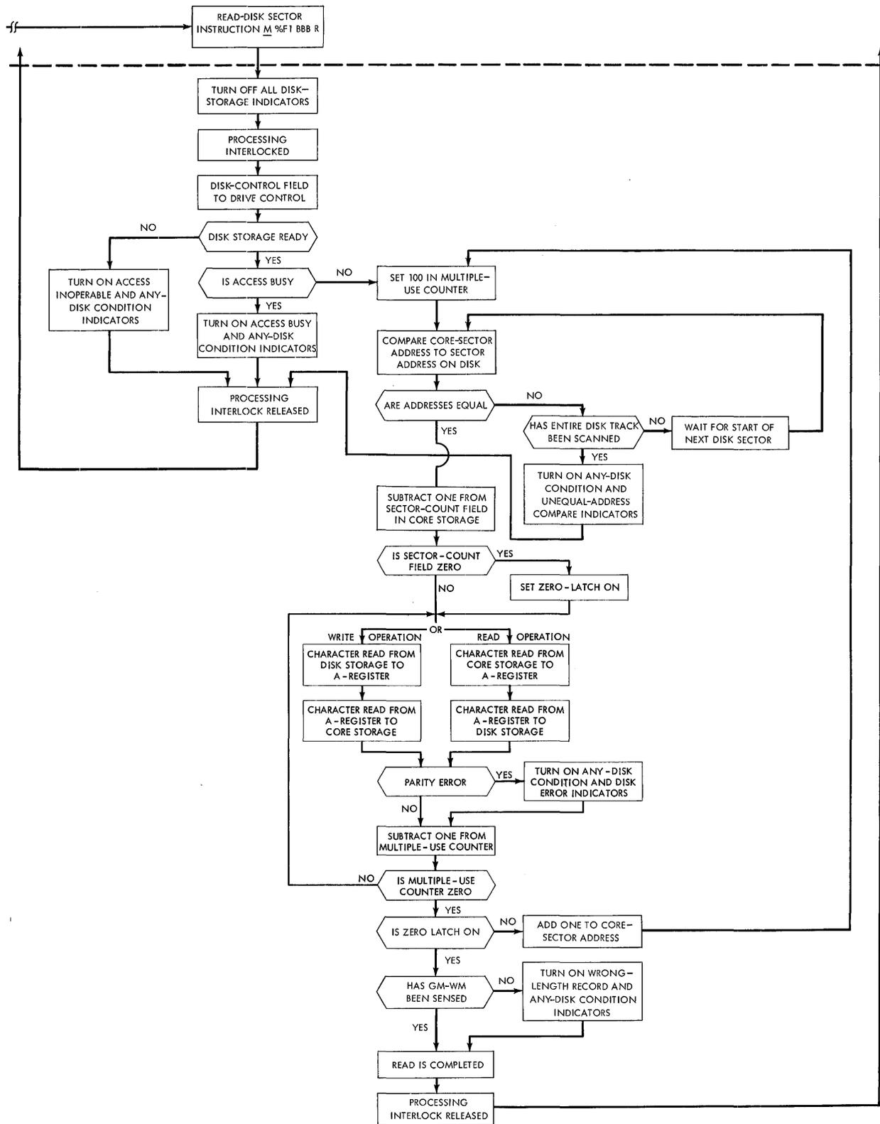
Figure G-19. Read/Write Disk Functional Schematic
