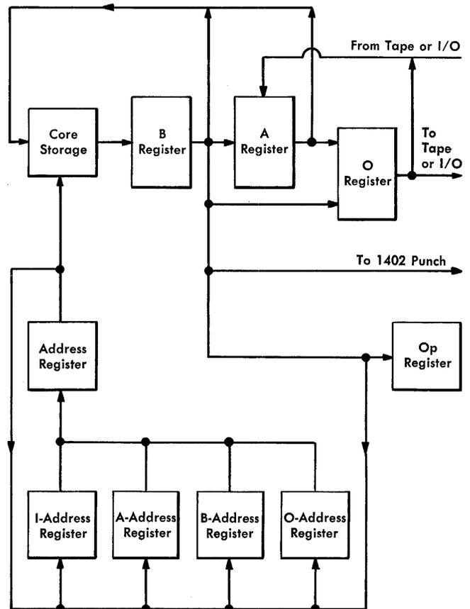
Figure I-54. IBM 1401 and 1460 Processing Overlap Data Flow
