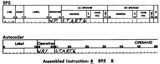
Figure I-105. Read-Punch Feed Write and Branch
