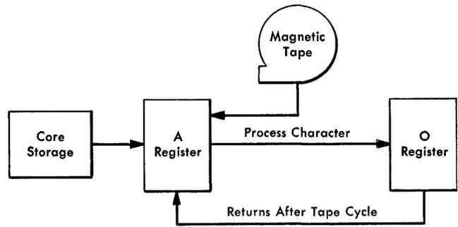
Figure I-56. Overlapped Magnetic-Tape Read Operation
