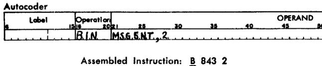
Figure I-23. Branch if Indicator On
