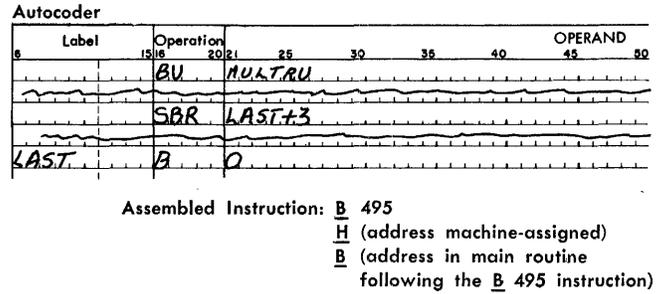
Figure I-4. Store Contents of B-Address Register (One Field)
