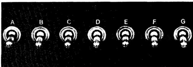
Figure I-84. Sense Switches
