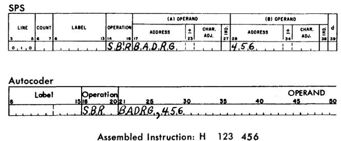
Figure I-5. Store Contents of B-Address Register (Two Fields)
