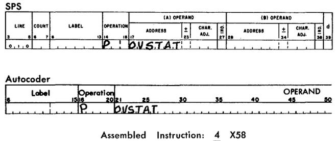
Figure I-69. Punch Card in Overlap Mode and Branch
