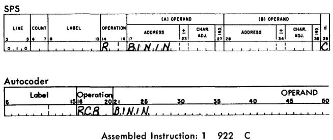
Figure I-9. Read Column Binary and Branch
