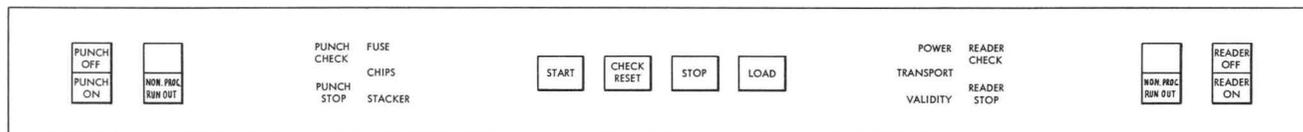
Figure 4. IBM 1402 Keys, Lights, and Switches (Models 1 and 3)
