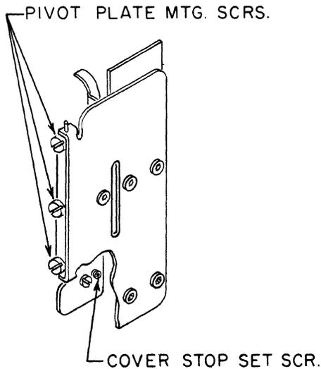
ADJUST FOR A CLEARANCE OF .048" TO .056"
