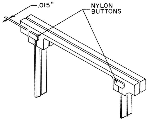
The button hammer assemblies must not be intermixed with non-button Hammer Assemblies 474805 (alpha-numeric) or 475486 (numeric), or increased hammer spring breakage may occur. Field changeover to the new assemblies is not necessary.
