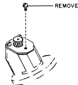
3. Add #22 grease through this tapped hole with a small diameter nozzleed grease gun extension (P/N 450566). Depress the plunger on the grease gun a sufficient number of times to force the grease out of the tapped hole or around the pinion gear.
