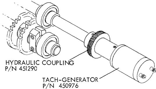
3. Ground the scope and connect vertical input and scope ground to Tach-Generator terminals.
