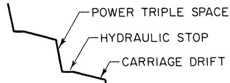
FIG. 12 BY-PASS ADJUSTED TOO TIGHT (1/4 TURN)
