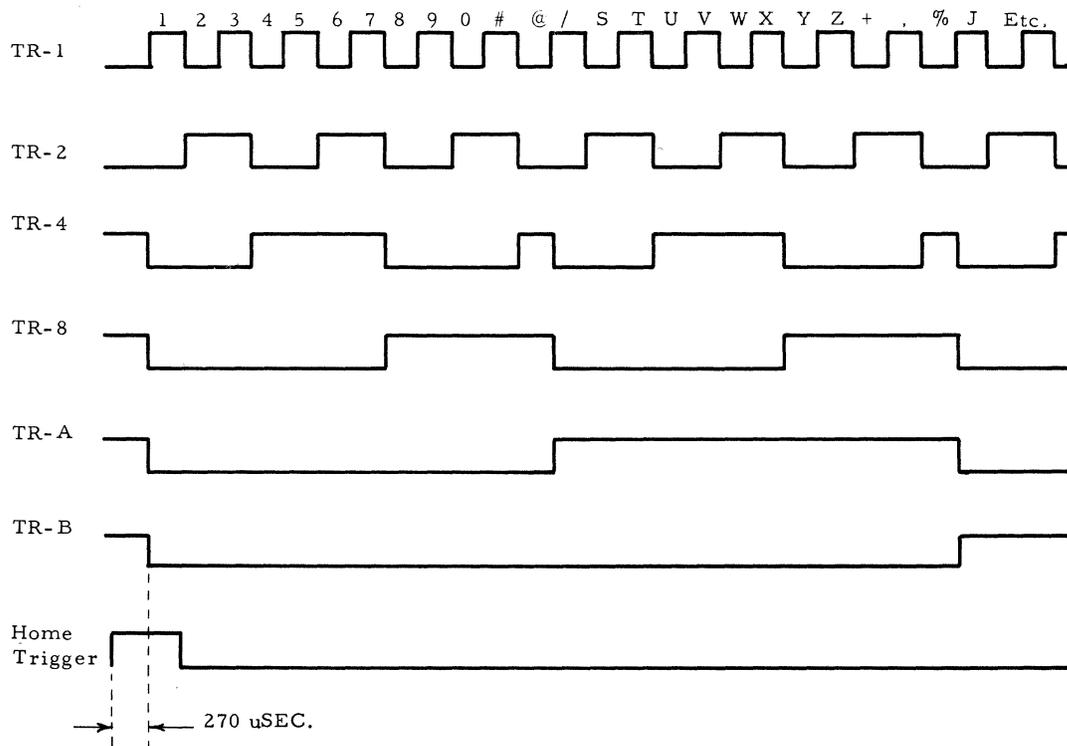
1. DO NOT PRINT: SYNC ON HOME TRIGGER GOING POSITIVE. COUNTER SHOULD ADVANCE BY 1 EVERY THIRD PSS PULSE (PSS PULSE ASSOCIATED WITH A SUB SCAN 1. PATTERN SHOULD BE AS SHOWN EACH DIVISION REPRESENTS 3 SUB-SCANS (1.65 MILLISECONDS).
