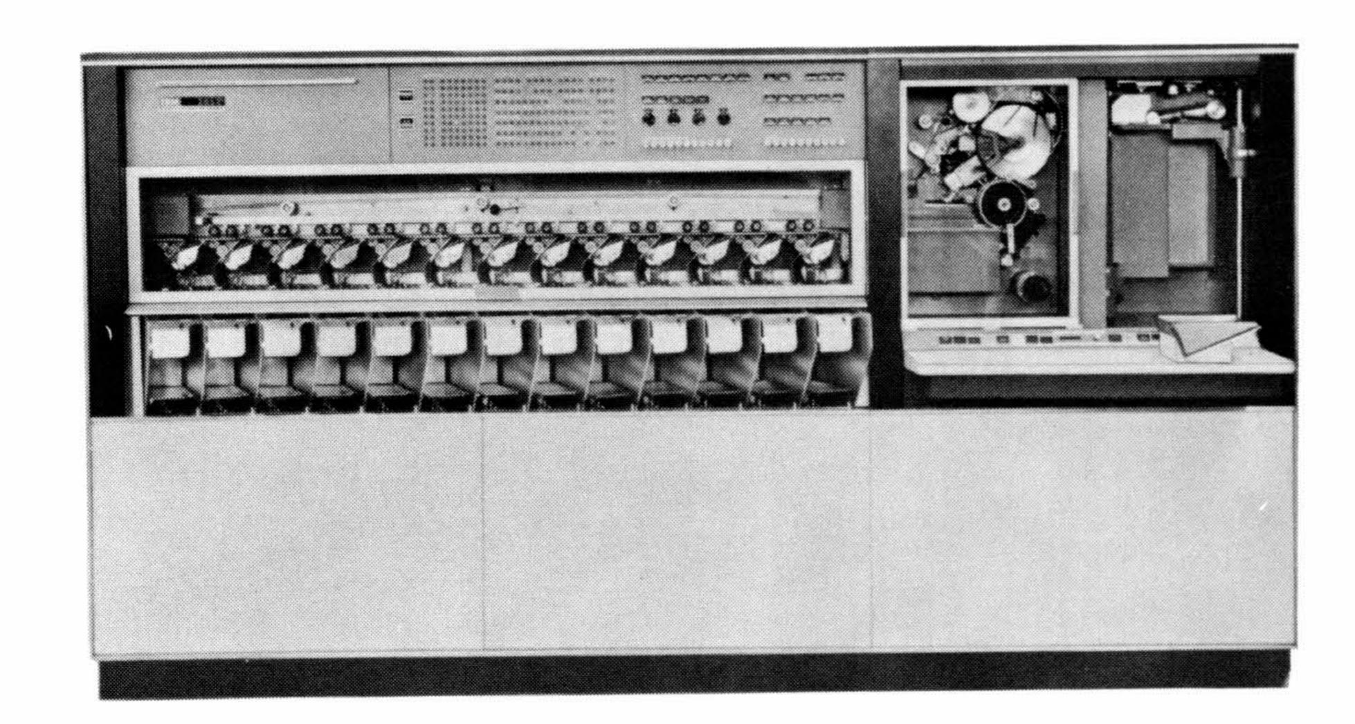
Flexibility of input is enhanced by the 1402 Card Read Punch. At rates of up to 800 cards per minute, stop-payment requests, new account data and off-cycle statement requests can be processed by the system. Thus while the 1410 continues processing, data can be added or deleted from customer records or special action can be initiated.
