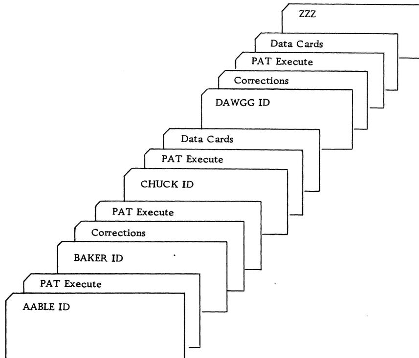
Figure 5. Object Program Corrections and Data Cards
