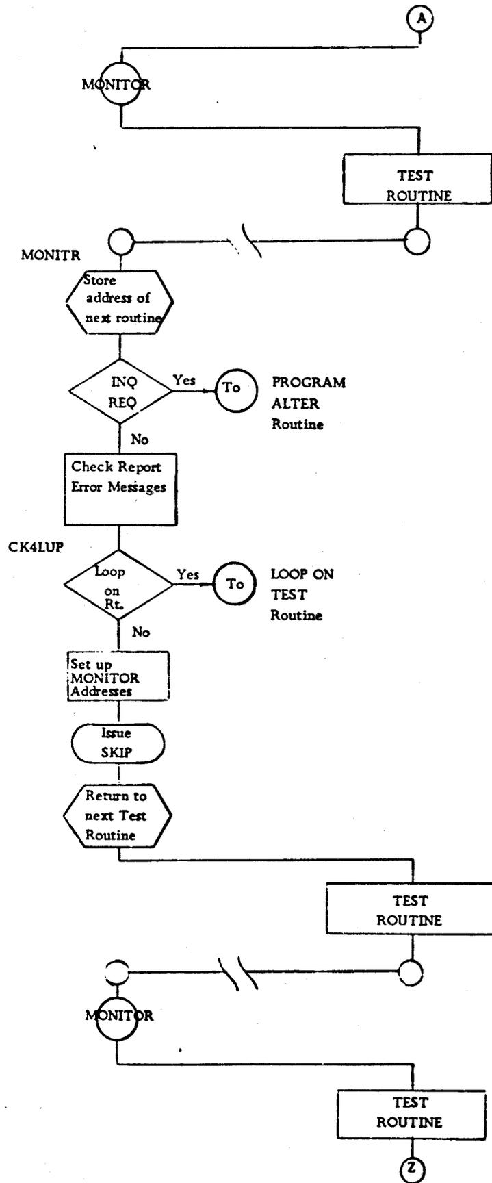
Sequence of Test Routines and common MONITOR Routine
