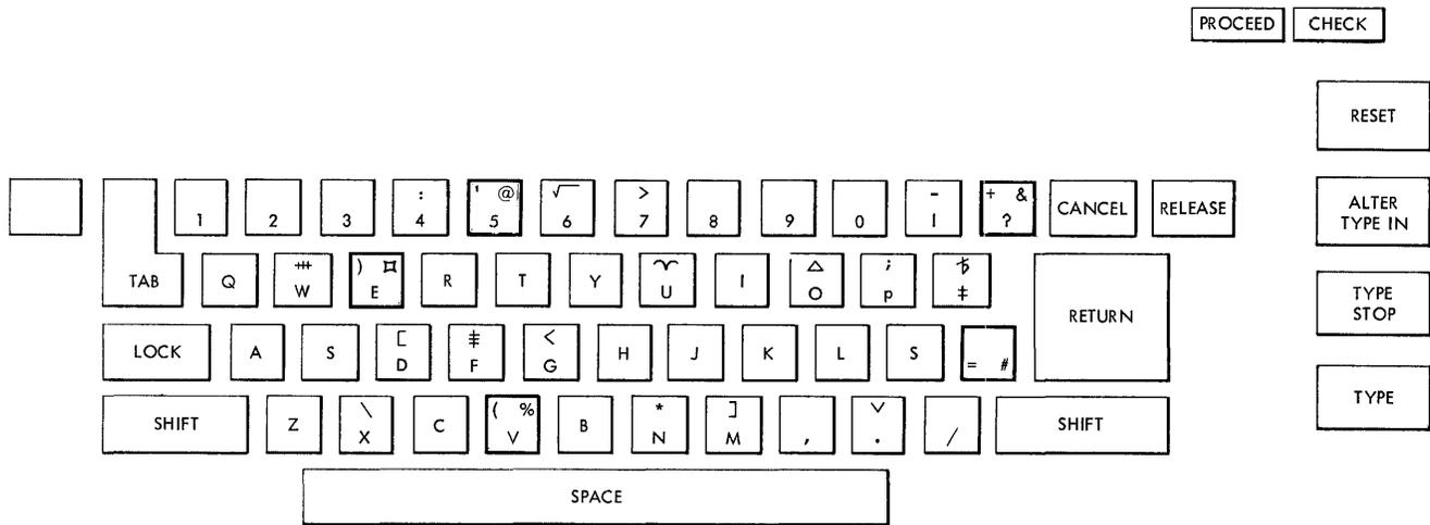
NOTE: Characters on left side of key are the H arrangement; characters on right side of key are the A arrangement.
