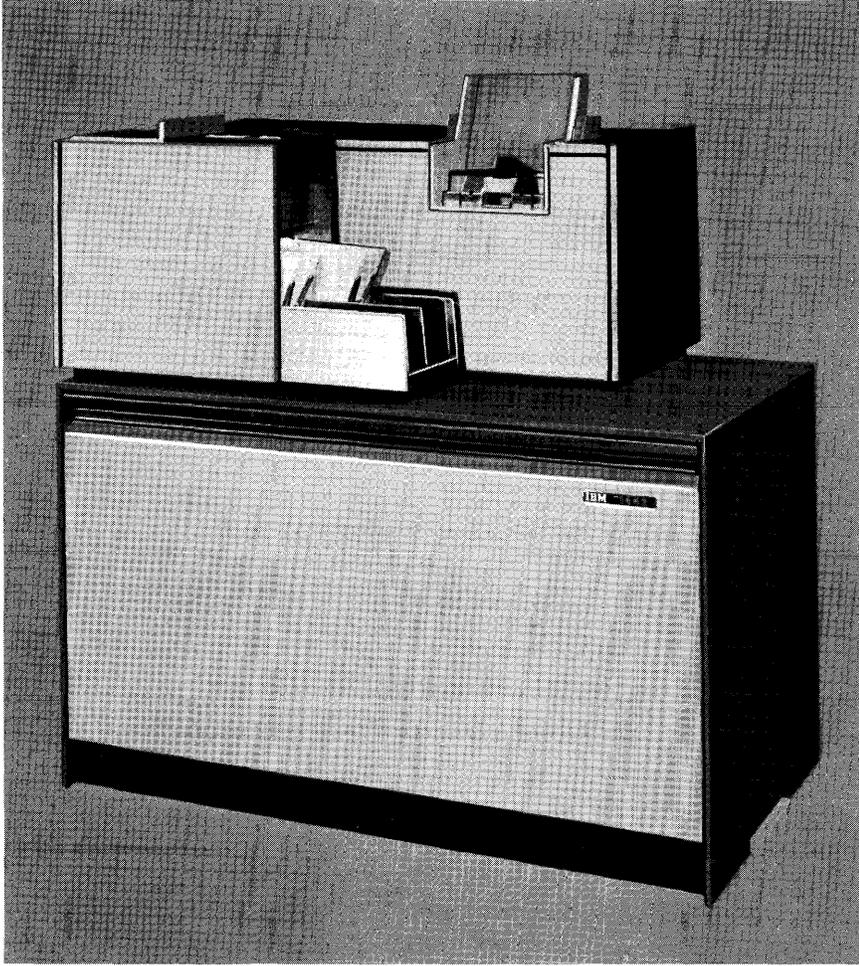
Figure 1. IBM 1442 Card Read-Punch
