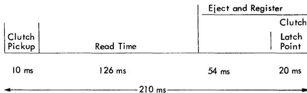
If 80 columns of a card are read and the Card Read instruction is given during the 20 ms at the end of the total card read cycle of 210 ms, then a rate of 285 cards per minute will be achieved. If less than 80 columns are read, there is commensurately more time available for computation.
