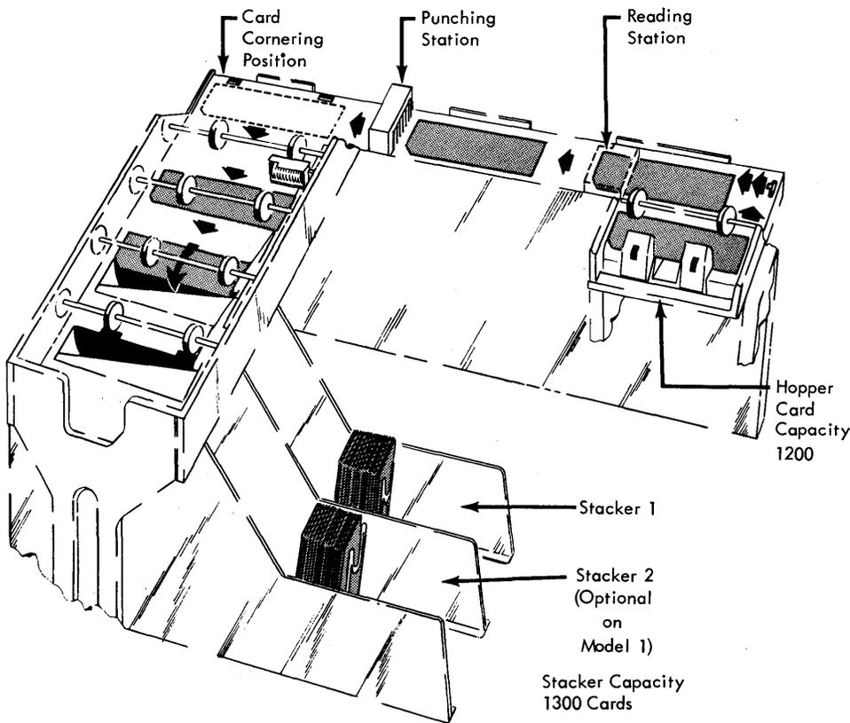
Figure 3. 1442 Card Feed and Punch Diagram
