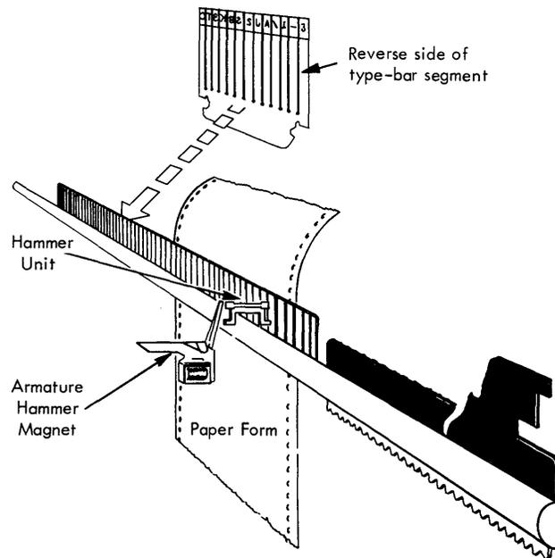
Figure 5. Printing Schematic
