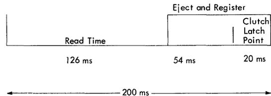
The above cycle is equivalent to a rate of 300 cpm. The formula to compute read time is now
