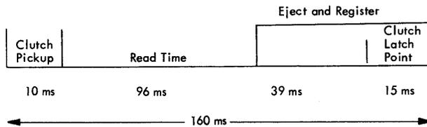
The basic cycle is 160 ms (equivalent to 375 cpm), which is reduced to 150 ms (400 cpm) if a card read instruction is given prior to the last 15 ms of the end of the card read cycle. Reading time for a card is given by the following formula:
