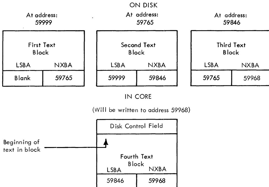
Figure 18. Working Storage text stream
