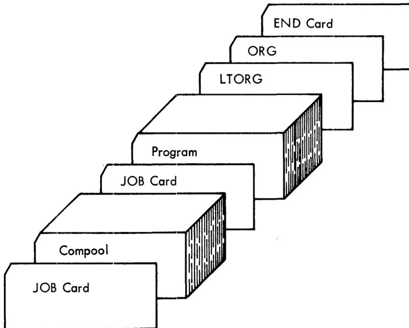
Figure 22. Source program decks ready to assemble
