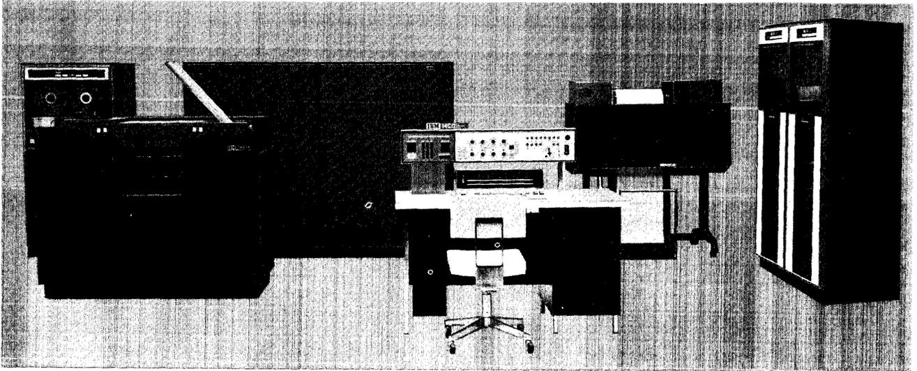
Figure 21. Tape-Oriented 1460 System
