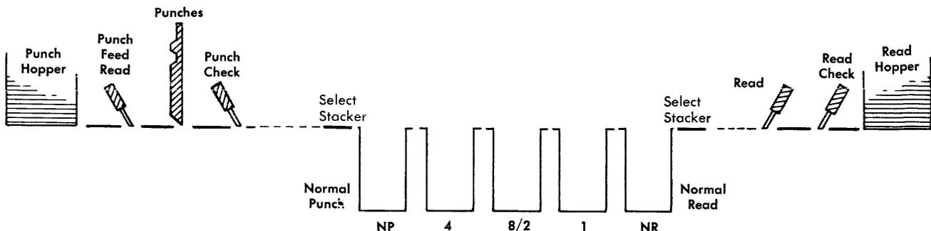
Figure 31. Punch-Feed-Read Schematic
