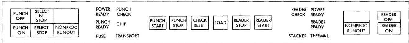
Figure 12. Switch, Key, and Indicator Light Panel
