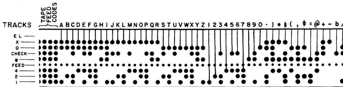
Figure 9. Paper Tape Tracks and Codes
