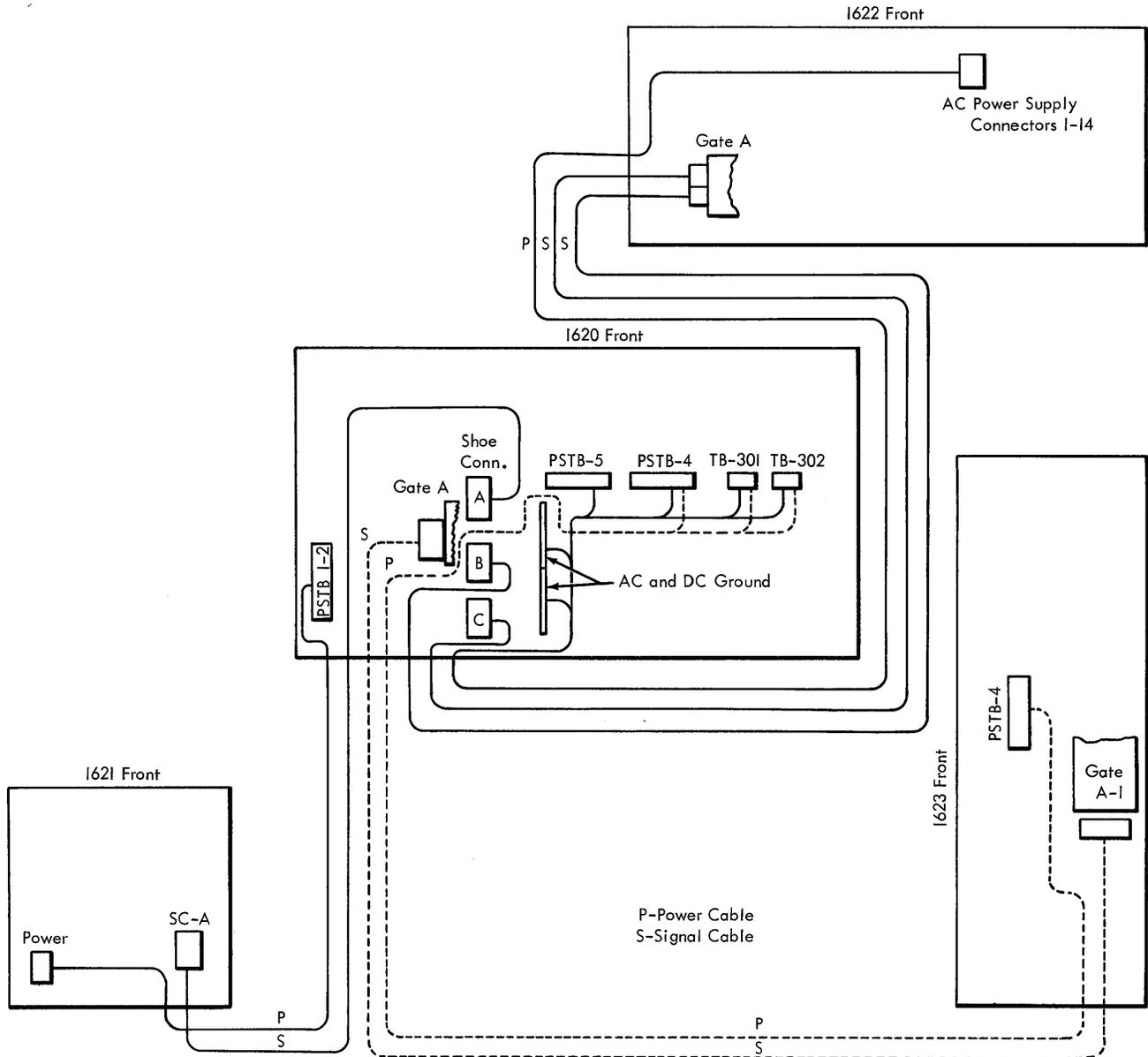
Figure 6. IBM 1620 Cable Connectors
