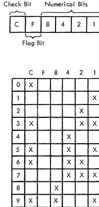
Figure 1. Bit Positions and Bit Configuration
