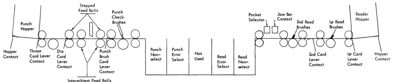
Figure 11. 1622 Feed Schematic
