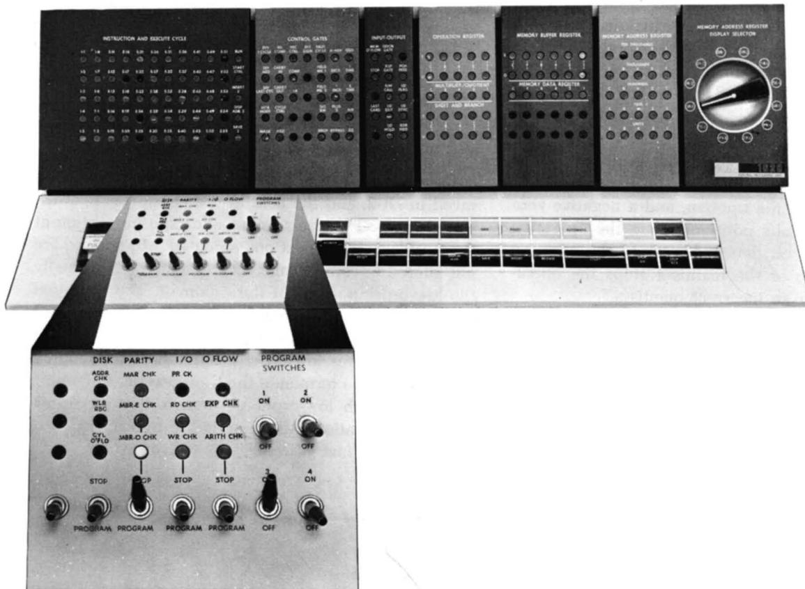
Figure 34. Indicators and Switches on 1620 Console
