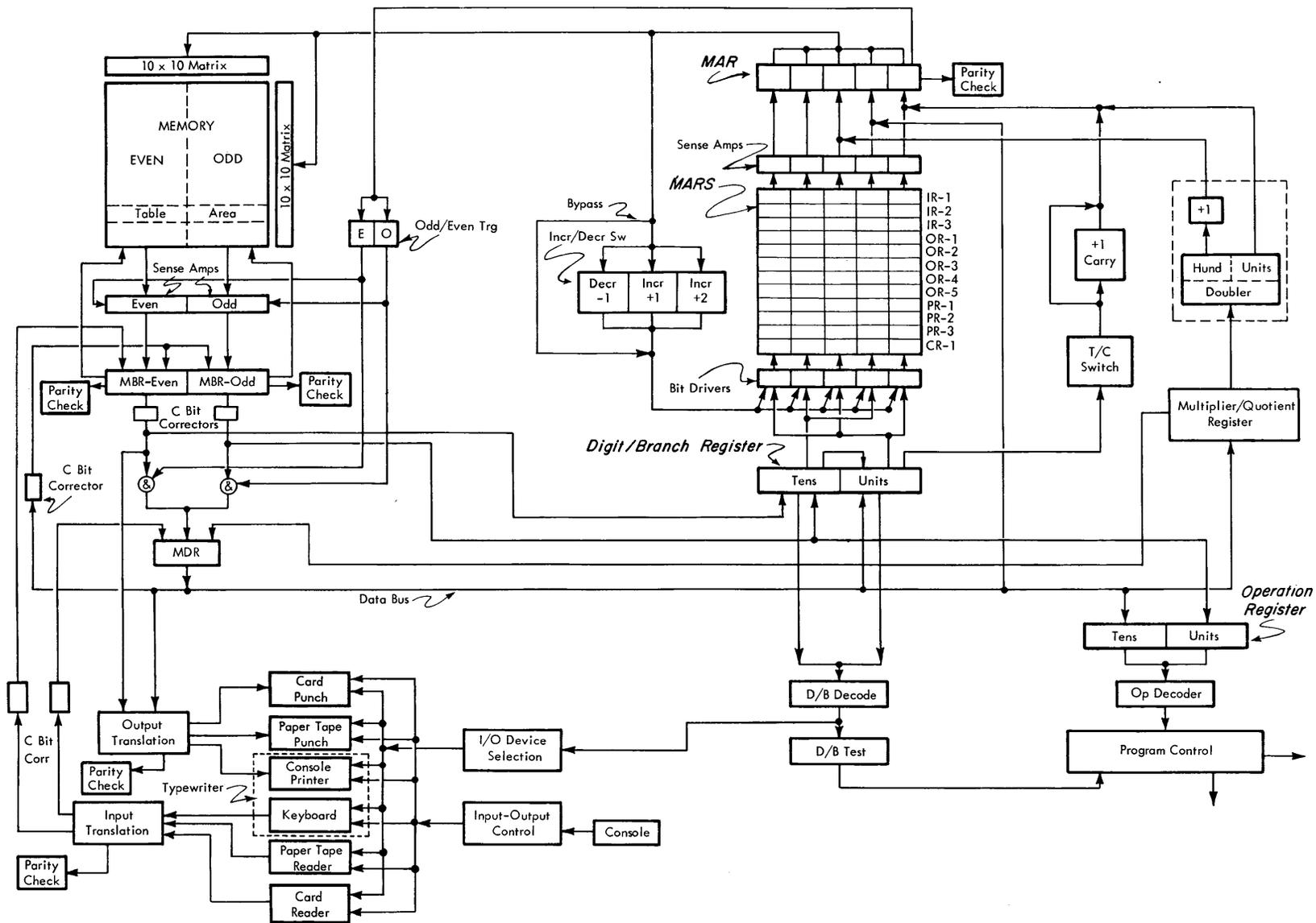
Figure 67. 1620 CPU Data Flow
