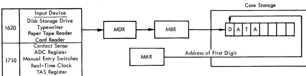
Figure 65. Data Flow of Input Operation
