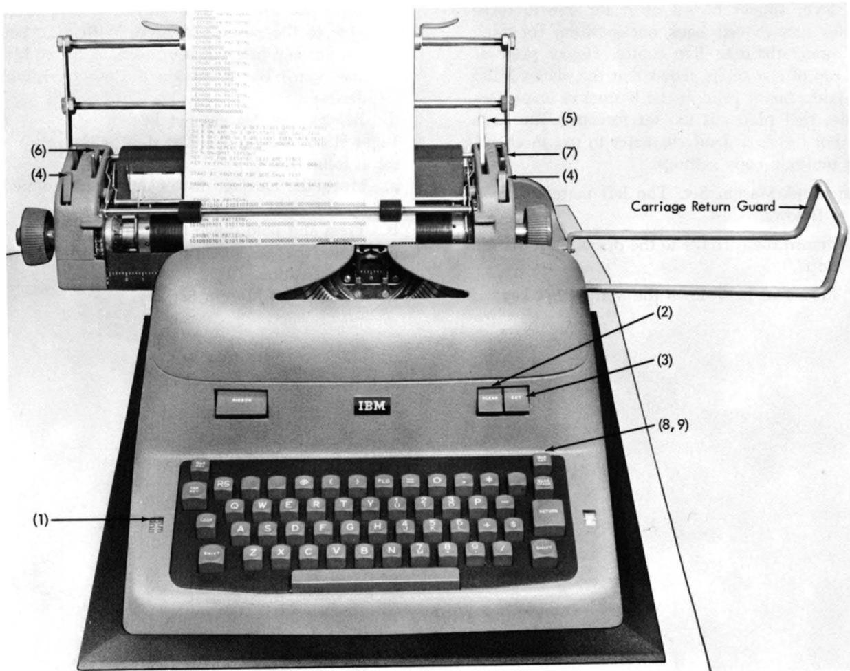
Figure 51. I/O Typewriter, Manual Controls and Keys
