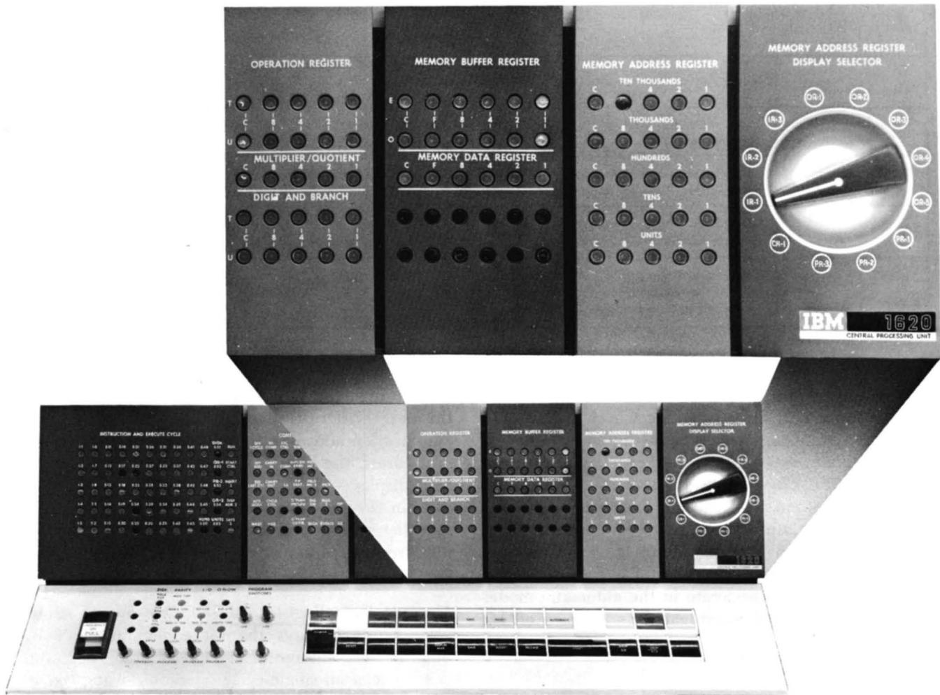
Figure 54. Register Display and Selector
