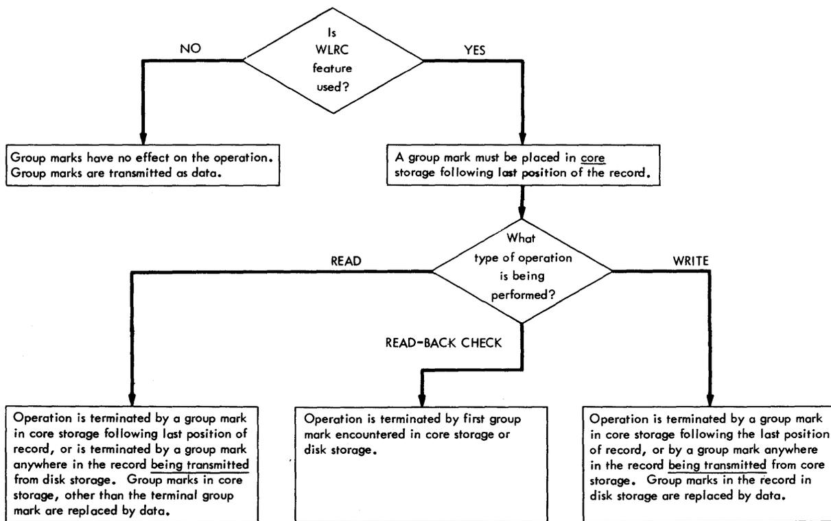
Figure 49. Effects of Group Marks on Disk Storage Operations
