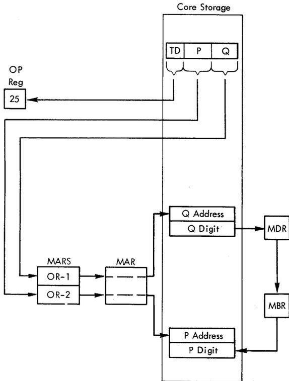
Figure 64. E Cycle of Transmit Digit Operation
