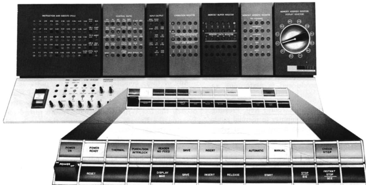
Figure 52. 1620 Control Keys and Signal Lights
