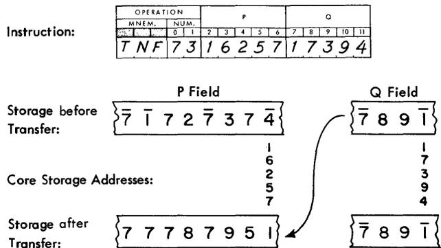
Figure 45. Transfer Numerical Fill
