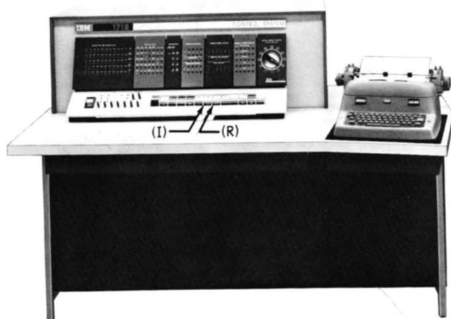
Figure 50. IBM 1620 CPU with I/O Typewriter
