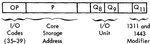
The  $Q_{11}$  position of the instruction is used to define 1311 operations and 1443 carriage spacing. Although the 1311 is controlled with standard input/output codes (36 and 38) and  $Q_{11}$  modifiers, the number and variety of instructions make their placement at the end of this section desirable.
