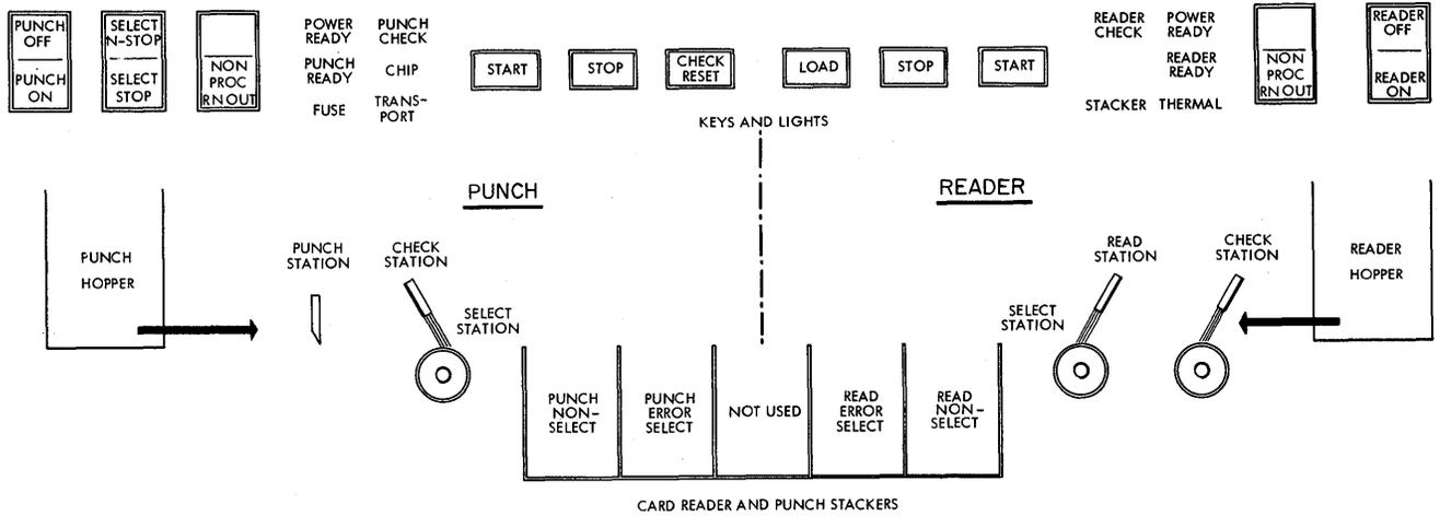
Figure 5. 1622 Keys, Lights, and Card Feed
