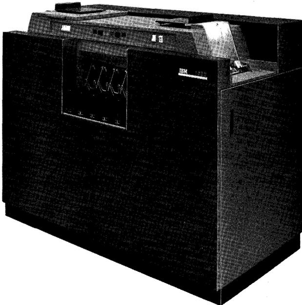
Figure 1. IBM 1622 Card Read-Punch
