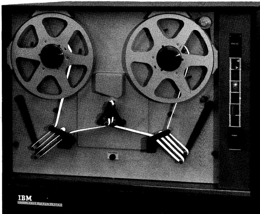
Figure 8. Paper Tape Reel Loaded
