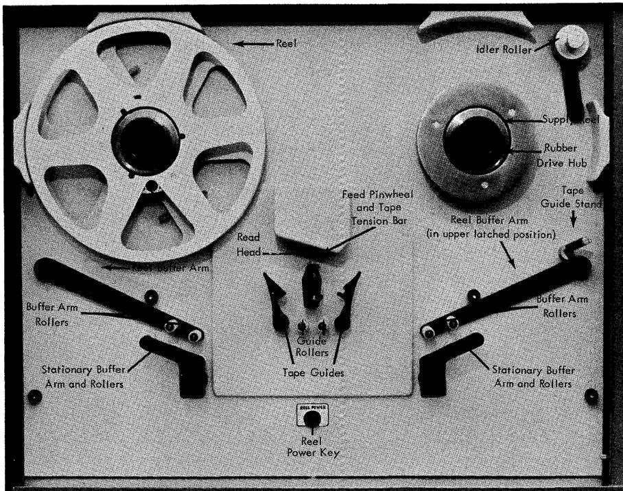
Figure 4. 1621 Tape Loading Area
