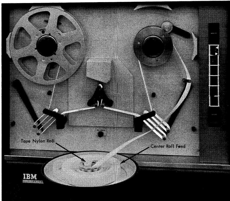
Figure 6. Center Roll Feed Loaded
