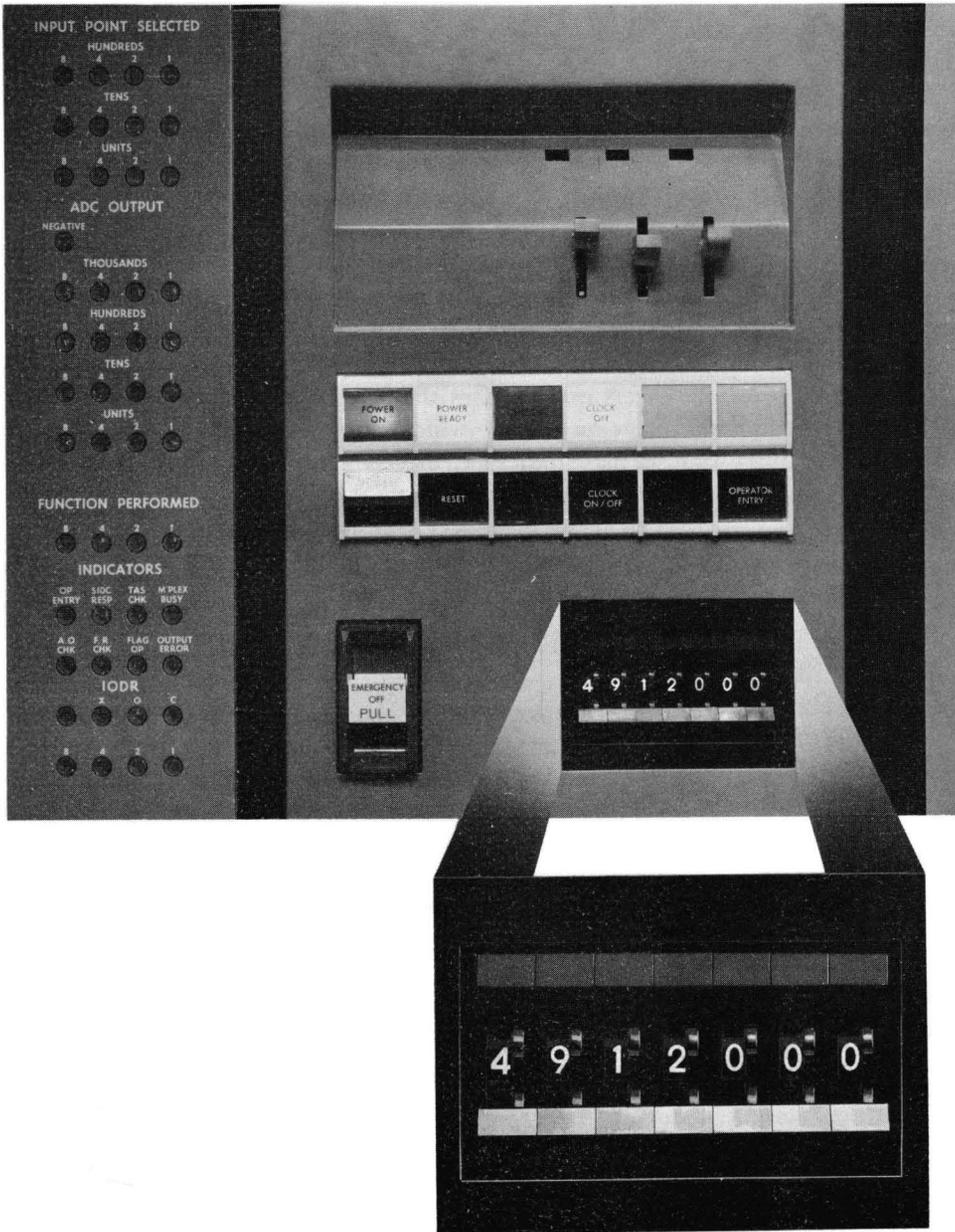
Figure 19. Manual Entry Switches, 1711 Operator's Panel
