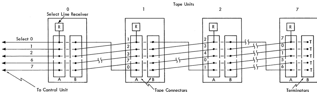
Figure 5. Rotation of Select (and Not Ready) Signal Lines
