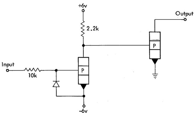
Figure 31. Tape Unit, Models 1-6, Line Driver
