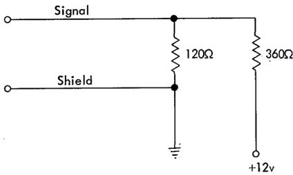
This is a representative circuit of those used in the terminator connector (part 5356195) which must be inserted in the connector B position of the last tape unit in a line. (Terminator part 5373693 would be used for tape units with simultaneous feature.)
