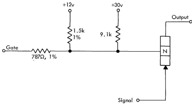
Figure 39. Simultaneous Preamp, Models 4-6 PE
