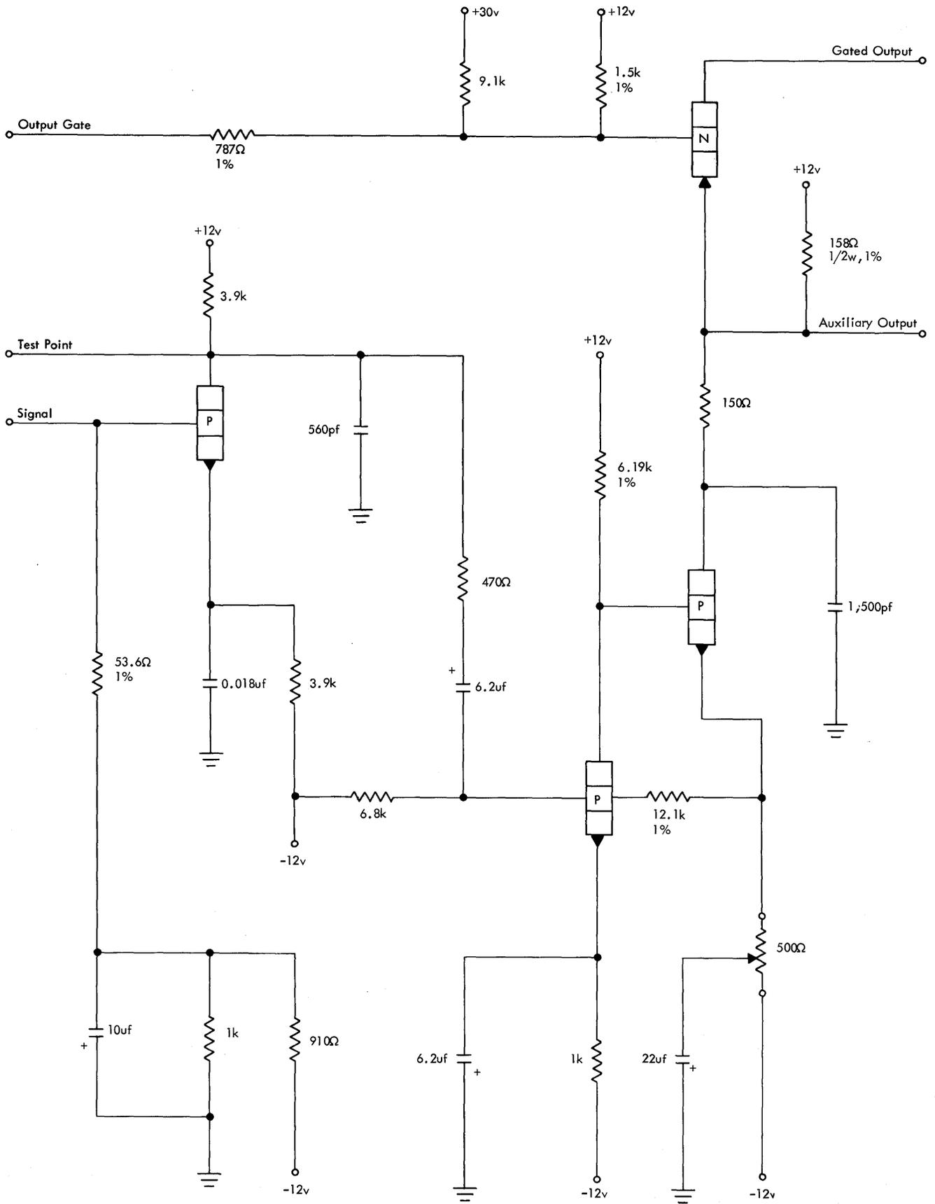
Figure 43. Tape Unit Read Preamplifier, Model 6 PE
