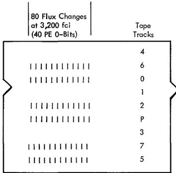
A PE tape mark is a special control block that consists of at least 80 flux reversals at 3,200 fci in data tracks P, 0, 2, 5, 6, and 7. Tracks 1, 3, and 4 are dc-erased. For recognition, the tape mark must contain at least 64 flux reversals in data tracks P, 0, and 5 (zone 1) or tracks 2, 6, and 7 (zone 2), with tracks 1, 3, and 4 (zone 3) dc-erased. Although the tape mark is preceded by approximately 3.75\* inches of erased tape, this gap is not a requirement.
