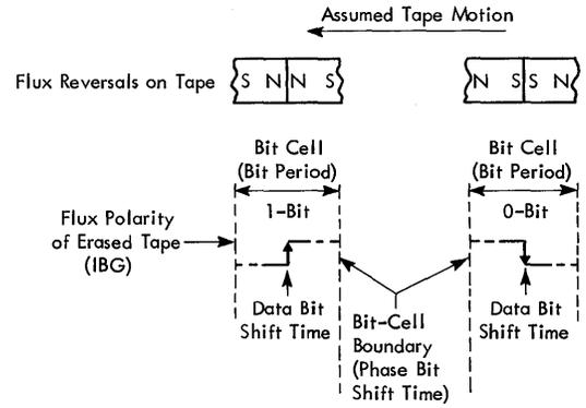
PE 1- and 0-Bits Defined (Tape Moving Forward)
