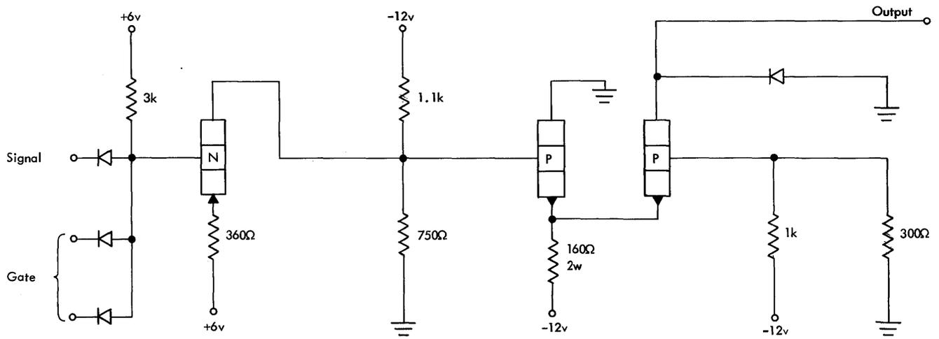
Figure 35. Control Unit, Model 2, Write Bus Driver
