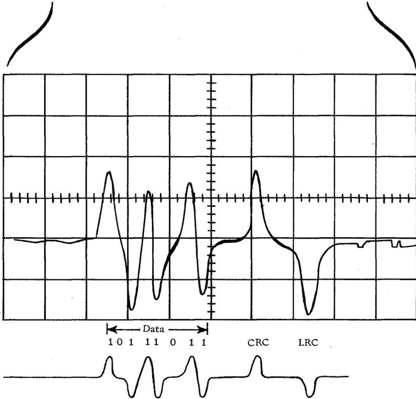
Figure 16. NRZI Read Bus Waveform (Nine Track)
