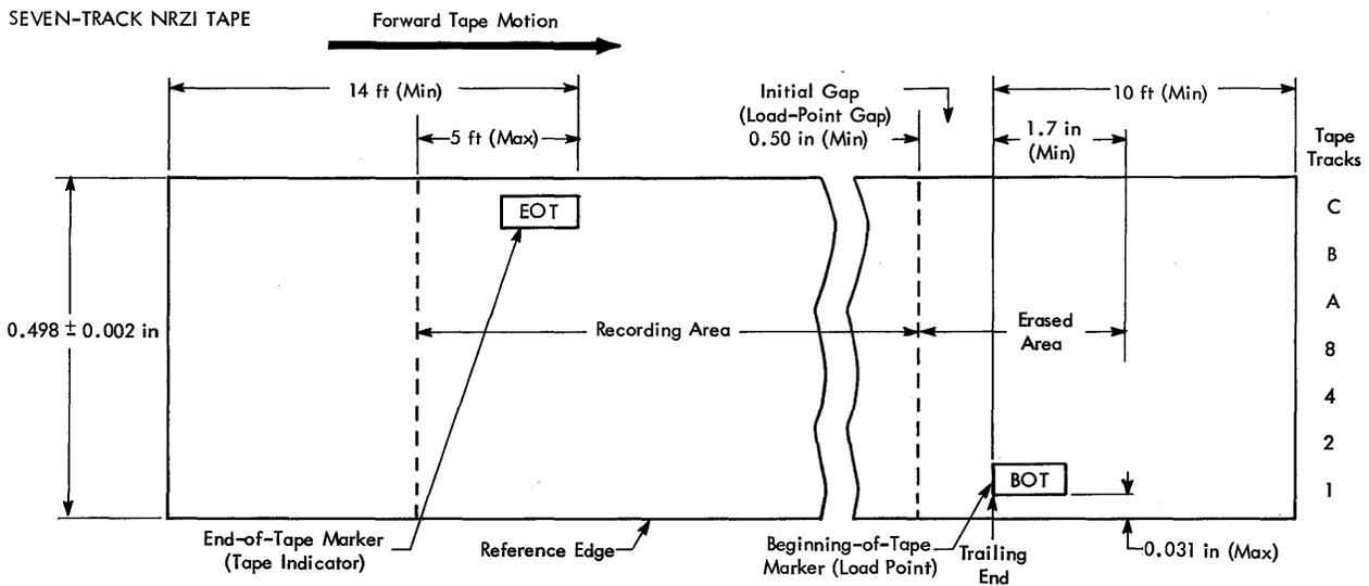
Note: Tape viewed from top while standing at front of tape unit. Markers are on top; recording is done on underside (oxide side) of magnetic tape.
