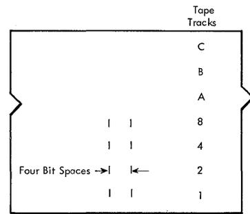
A seven-track NRZI tape mark is a special control block that consists of a character with 1-bits in data tracks 8, 4, 2, and 1, and an identical LRC character four bit spaces from it. Although the tape mark is preceded by approximately 3.90\* inches of erased tape, this gap is not a requirement.
