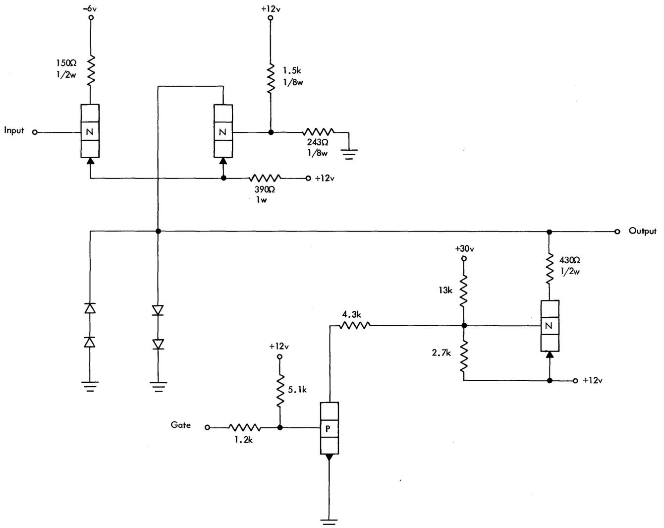
Figure 36. Tape Unit, Models 4-6, Write Bus Receiver
