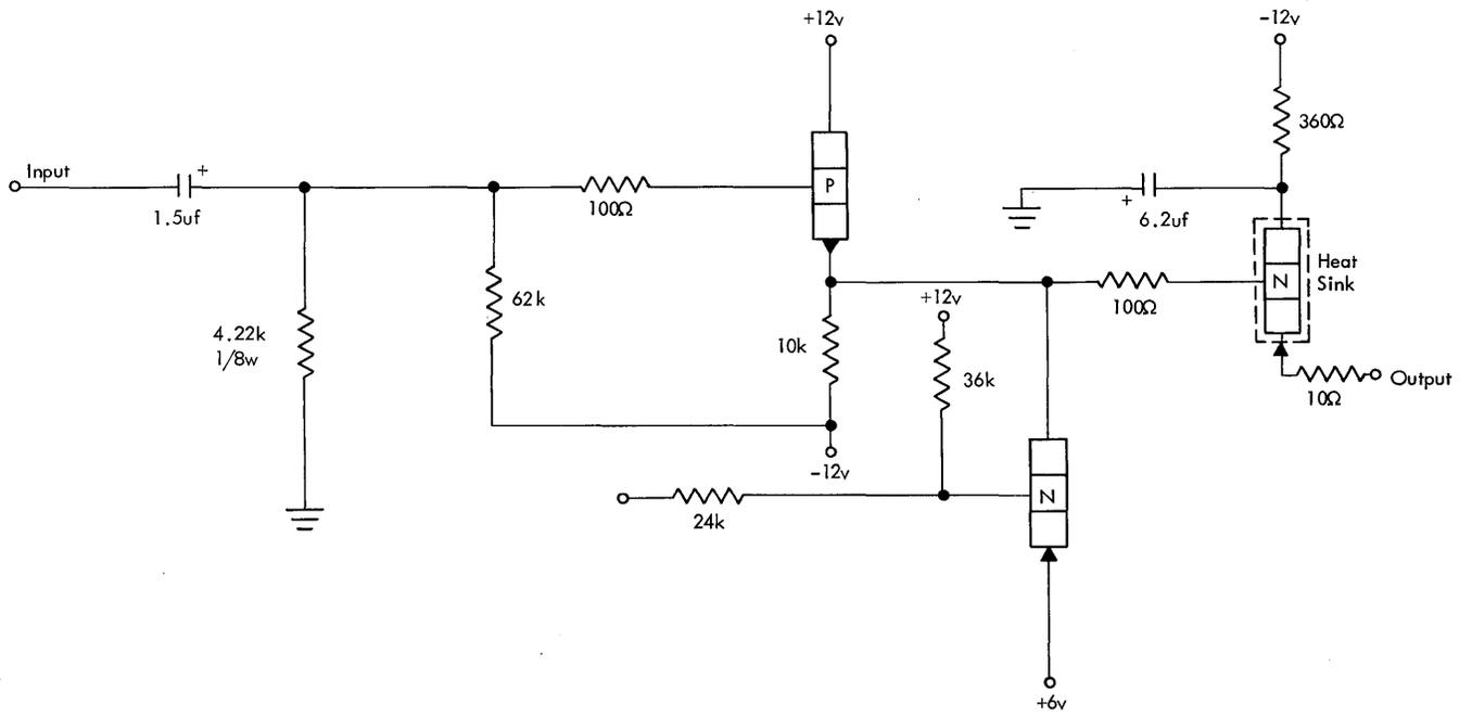
Figure 38. Simultaneous Preamp, Models 4-6 NRZI
