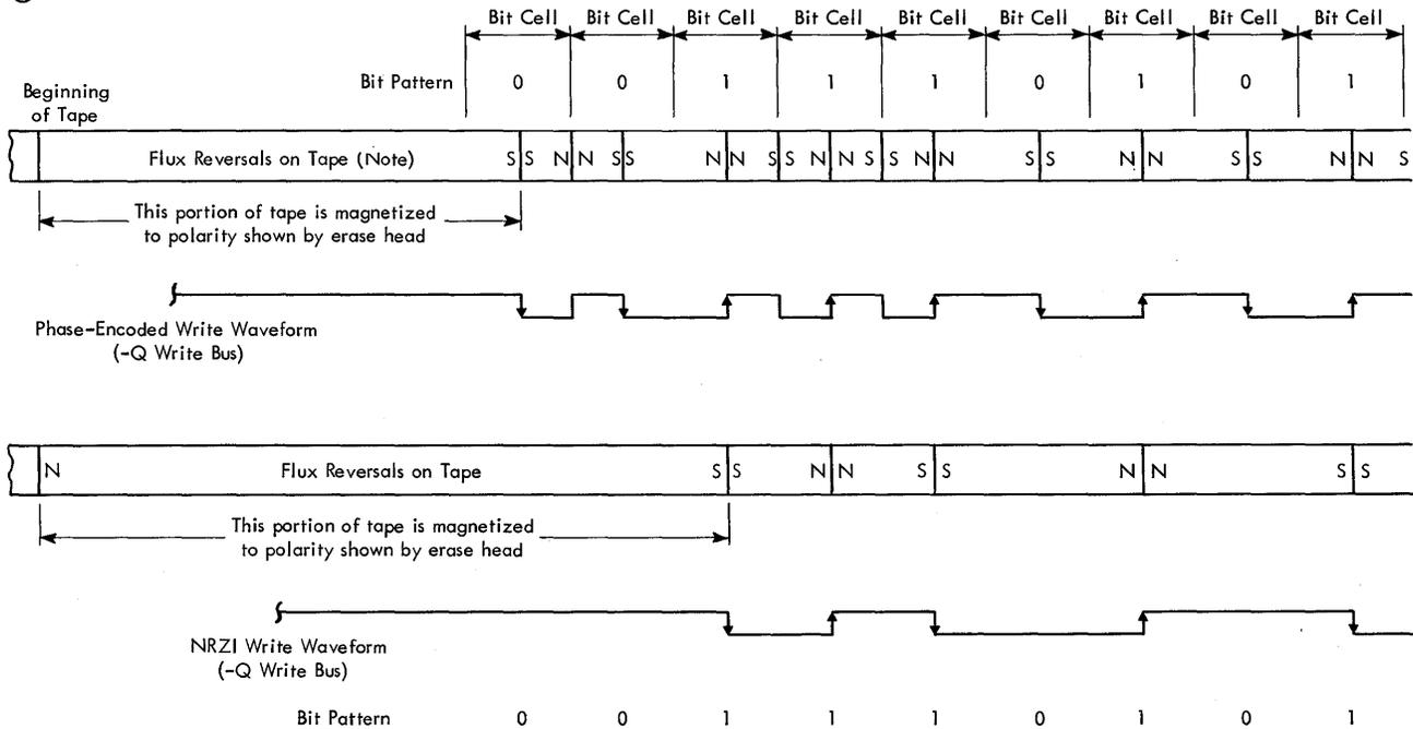
**Note:** A flux reversal (NN or SS) is the area where the flux polarity of the magnetized tape is reversed. The particles of oxide coating on the tape are magnetized by the write head to act like tiny magnets whose combined effect is shown in this figure.
