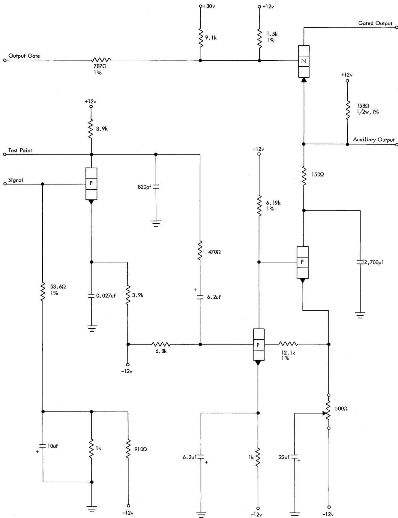
Figure 42. Tape Unit Read Preamplifier, Model 5 PE
