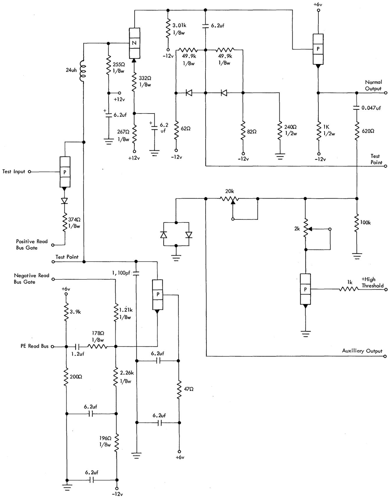
Figure 44. Control Unit, Model 2, Read Bus Receiver PE
