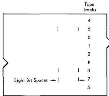
A nine-track NRZI tape mark is a special control block that consists of a character with 1-bits in data tracks 3, 6, and 7, and an identical LRC character eight bit spaces from it. No CRC character is written. Although the tape mark is preceded by approximately 3.75\* inches of erased tape, this gap is not a requirement.
