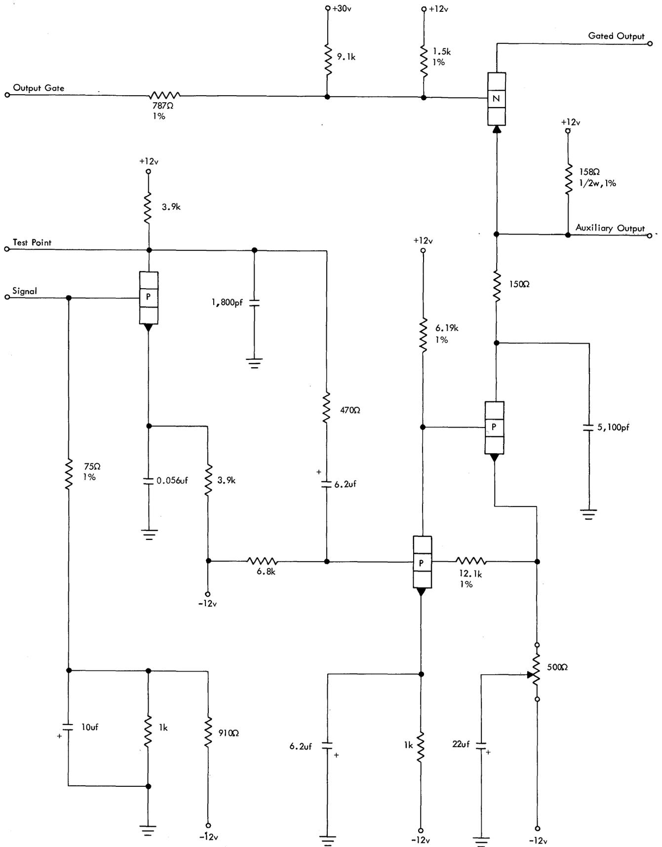
Figure 41. Tape Unit Read Pre-amplifier, Model 4 PE
