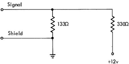
Figure 29. Write Bus Terminator, Models 4-6
