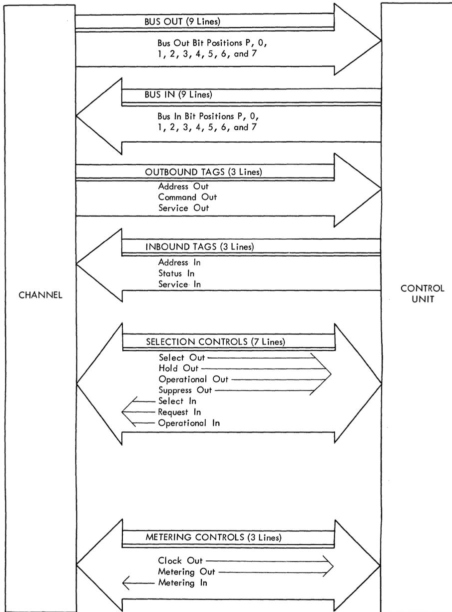
FIGURE 1-5. INPUT/OUTPUT INTERFACE LINES, SYSTEM/360
