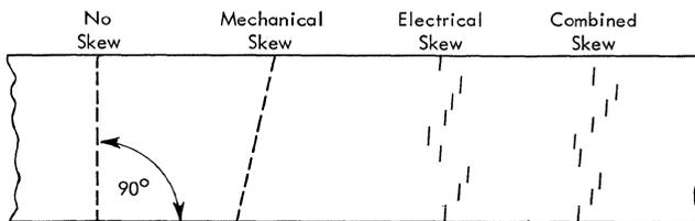
FIGURE 1-3. WRITE SKEW (EXAGGERATED)
