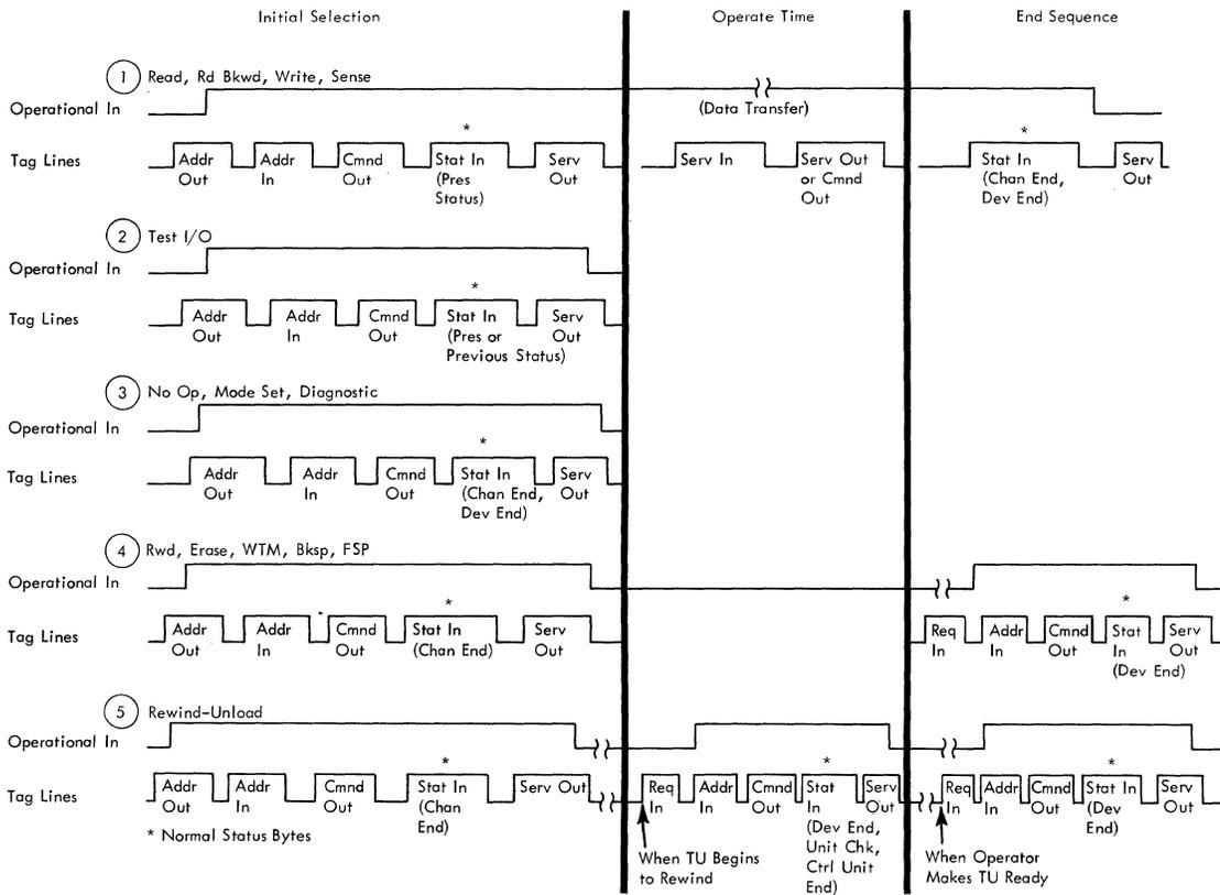
FIGURE 1-10. CHANNEL INTERFACE TAG LINE SEQUENCES
