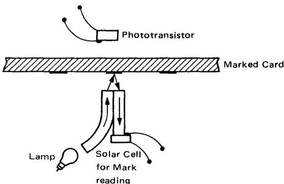
Figure 3. Hole Reading and Mark Reading [06503]
