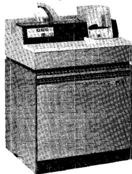
2. *IBM 2501 Card Reader Models B1 and B2* connected to System/360 Model 25, 30, 40, 44, 50, or 65 via the standard interface.
