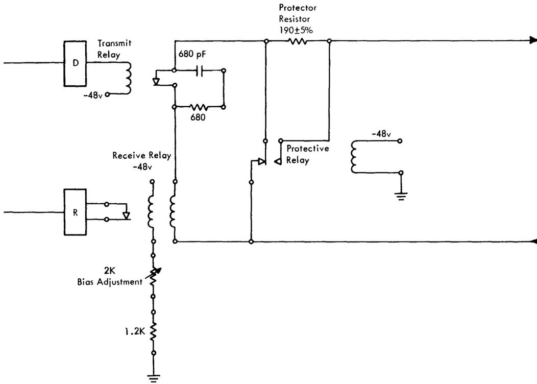
Figure 7. Telegraph Adapter Interface
