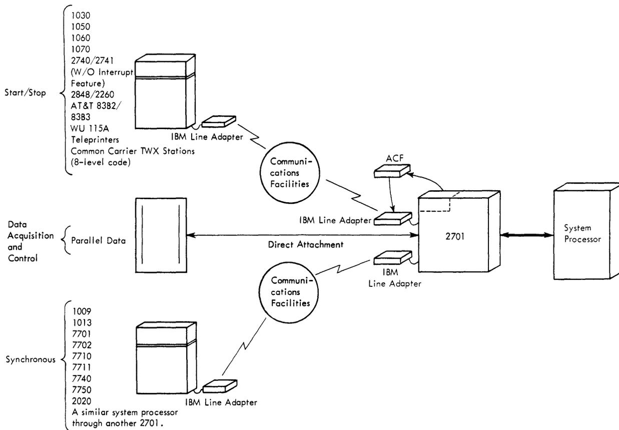
Figure 1. 2701 in a System Environment
