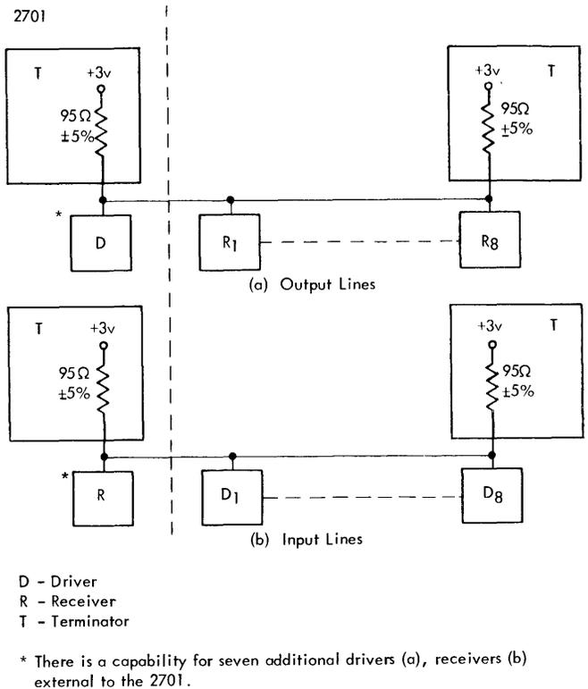
Figure 15. Input and Output Terminations
