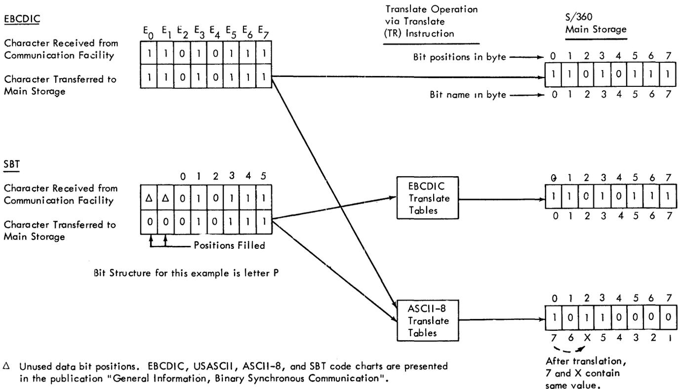
Figure 12. Code Translation of a Received Character (to EBCDIC or ASCII-8)
