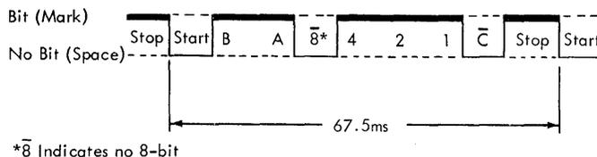
Figure 5. Bit Configuration of a "G" Character (Serialized)
