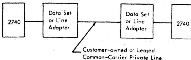
Figure 6. Point-to-Point, Terminal-Terminal
