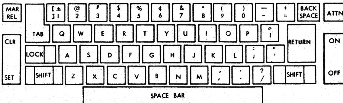
Note: When this keyboard and associated print elements are specified, the line code assignments of the graphic characters change and are not compatible with the PTT/BCD and PTT/EBCD print elements and associated keyboards.
