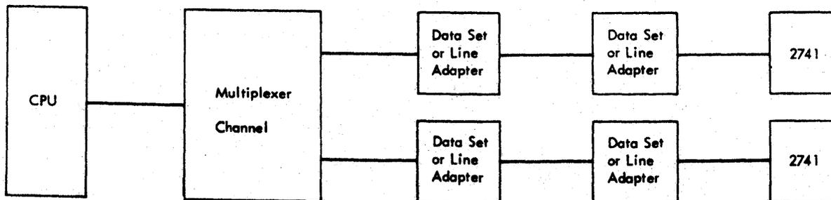
Figure 22. IBM 2741 Point-to-Point
