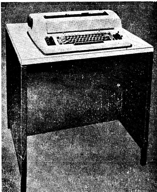
Figure 1. IBM 2740 Communication Terminal
