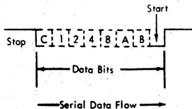
Figure 10. IBM 2740/2741 Data Flow
