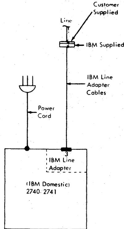
Figure 18. IBM 2740/2741 Cables
