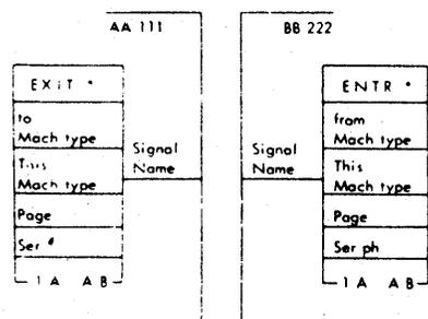
**Cable Logic Blocks:** Two logic blocks (Figure 56) are used to define each cable: one logic block shows the "from" location; the other logic block shows the "to" location. Line 1 contains CABL\* for regular cables (both intergate and intragate) and XOVR\* for crossover cables.
