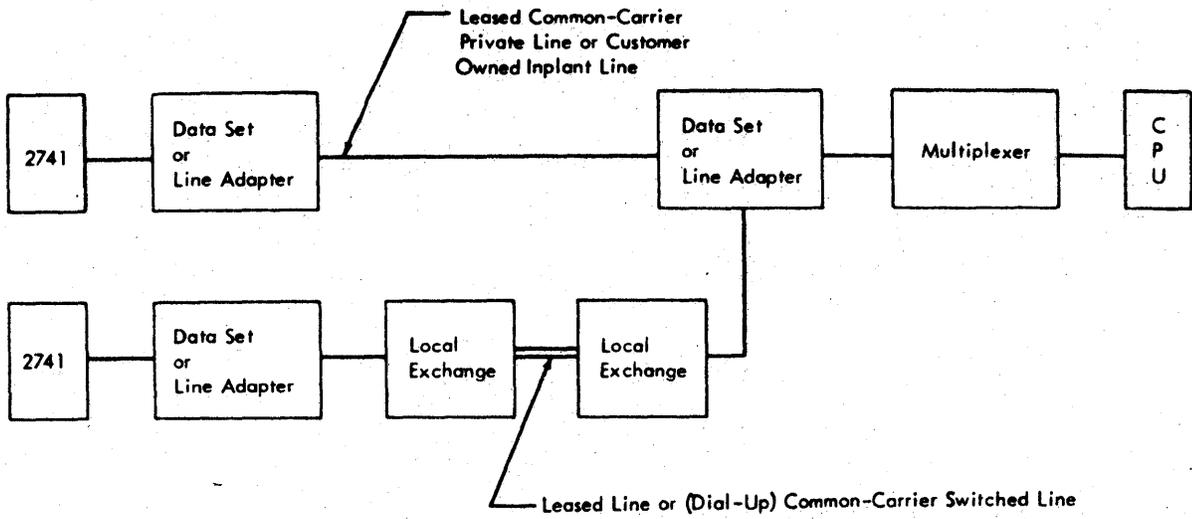
Figure 7. Point-to-Point, Terminal-Computer
