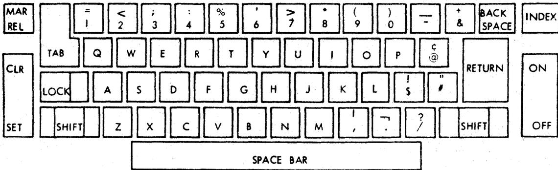
Figure 5. IBM 2740 Keyboard (PTTC/EBCD)
