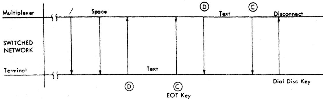
Figure 30. Transmit Control (without Checking Special Feature)
