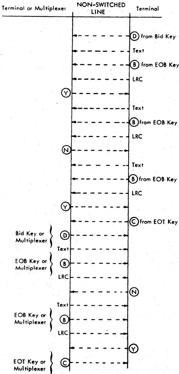
Figure 26. Point-to-Point Operation (with Checking Special Feature)
