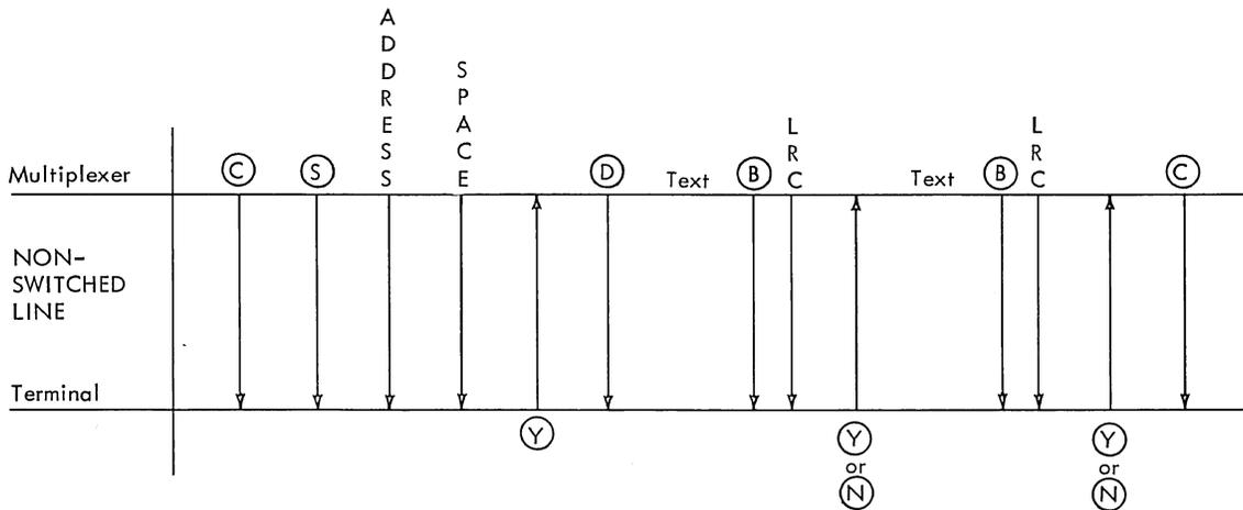
Figure 34. Station Control, Multiplexer Addressing (with Checking Special Feature)
