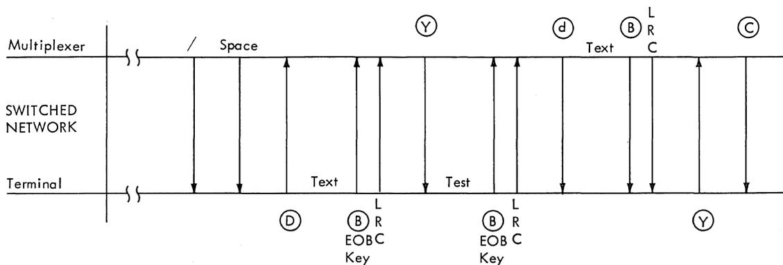
Figure 31. Transmit Control (with Checking Special Feature)
