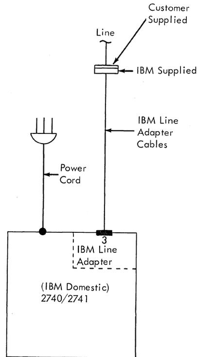
Figure 18. IBM 2740/2741 Cables
