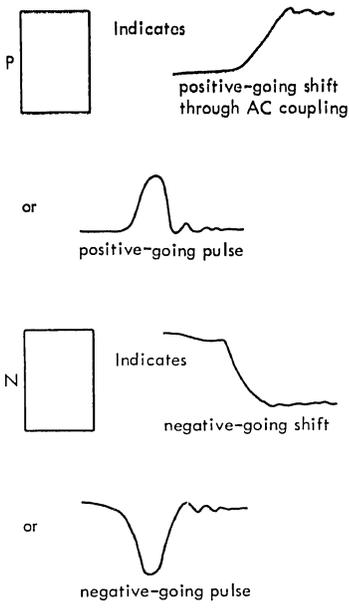
Figure 43. Capacitive Inputs
