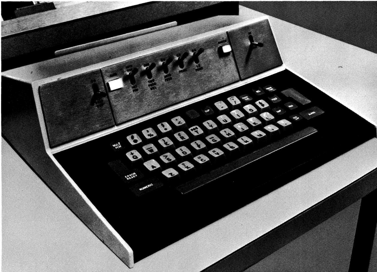
Figure 545-8. Sixty-Four Character Keyboard and Controls (EL Arrangement)
