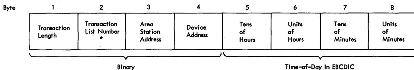
\* Left-hand rotary switch setting is referenced to the user transaction tables, and the transaction list number from the table is placed in byte 2 of the header.
