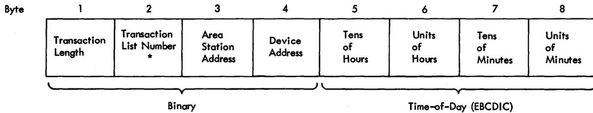
\* Upper left-hand rotary switch references a transaction from the user's transaction table. The transaction list number from the table is placed in byte 2 of the header.
