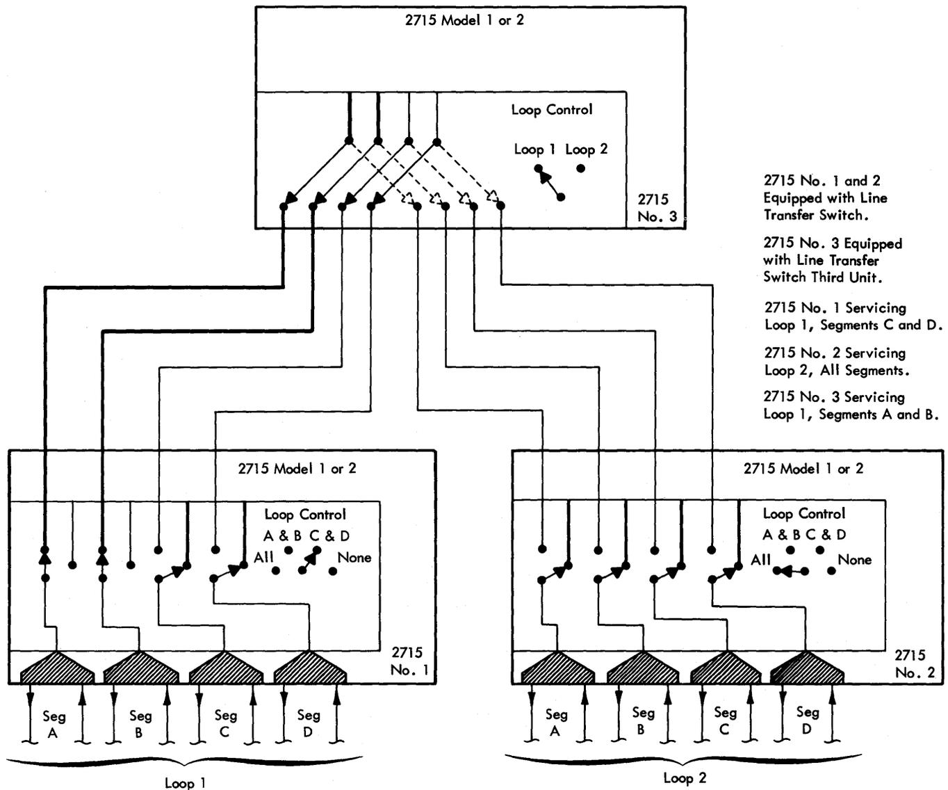
Figure 19. Line Transfer Switch—Third Unit
