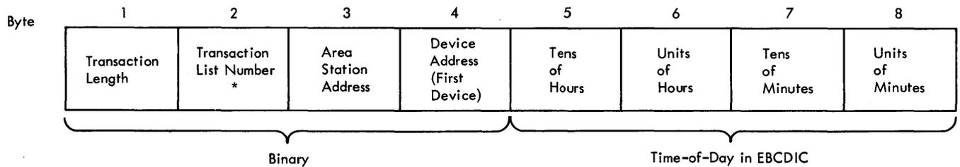
\* The Transaction Selection Switch position is referenced to the user transaction table. The transaction list number from the table is placed in byte 2 of the header.
