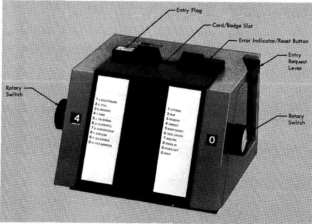
Figure 3. IBM 2795 Data Entry Unit
