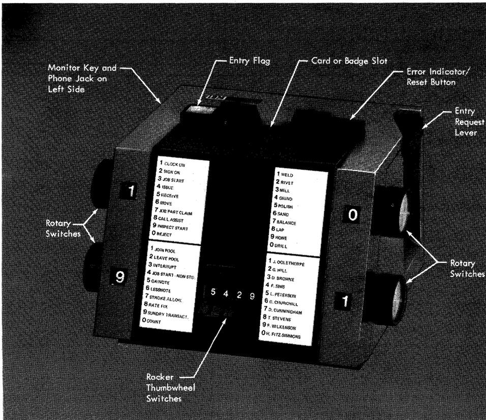
Figure 4. IBM 2796 Data Entry Unit
