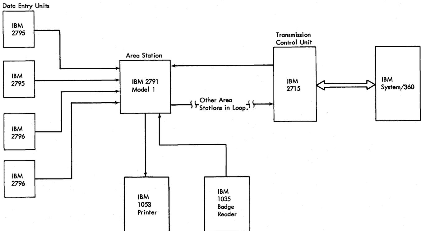
Figure 1. A Typical IBM 2790 Data Communication System
